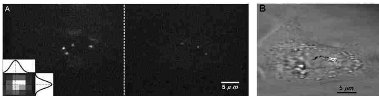
Figure 2.7. Example of Single QD-EGF Tracking. A) Images from one frame of two-color QD-EGF tracking on the surface of SKBR3 cells showing each channel (QD655 on the left, QD585 on the right) as projected by the Optosplit. Inset on the lower left shows the PSF fits of a single QD655. These images were acquired with excitation intensity of 4.7 \text{ W/cm}^2 (436/10 BP), results in average photon counts of 314 and 172 for QD655 and QD585, respectively. The localization error is then 24 nm for QD655 and
