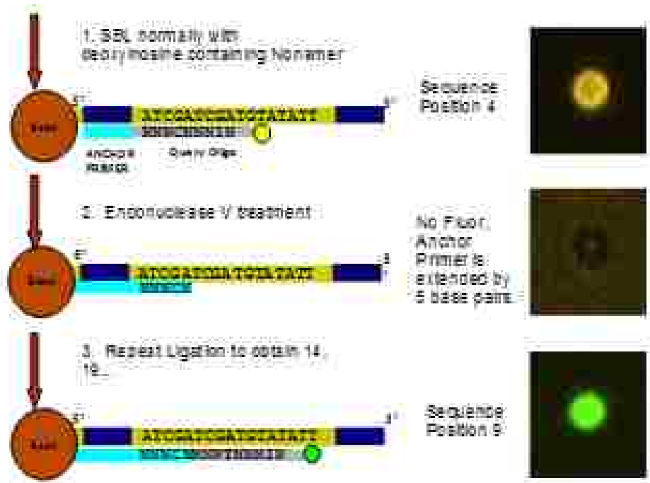
Figure 7. Sequencing By Ligation with Endonuclease V Digestion. 1) Sequencing the fourth base in the template tag, by using standard SBL with a Query Oligo that contains a Deoxyinosine (I). 2) Endonuclease V will recognize the Deoxyinosine and cleave the second phosphate bond towards the 3' end. The picture has white light background to make the bead visible as all fluorescence is ablated. 3) Repeat SBL to obtain the next positions.
