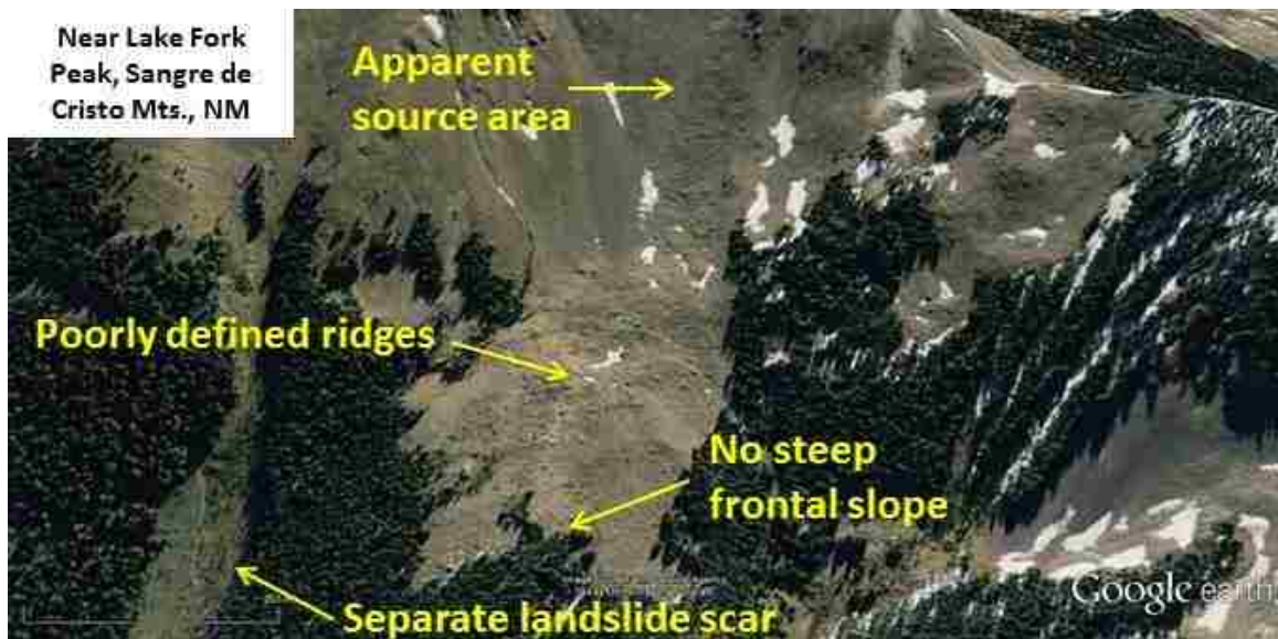
Figure 3.7 Landslide deposit in the Sangre de Cristo Mountains. Source: Google, NAIP 2011
