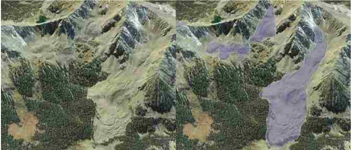
Figure 3.10 Rock glacier digitization in the Sangre de Cristo Mountains. At least five rock glaciers are evident in the image to the left. Three of the five rock glaciers are in contact with each other and combined into one contiguous polygon in the image on the right (left most polygon). Source: Adapted from Google, NAIP 2013
