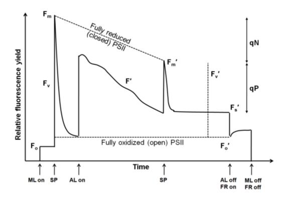
Figure 2.4: Nomenclature of PAM fluorescence parameters for dark-adapted leaf [Mac neill, 2011].
