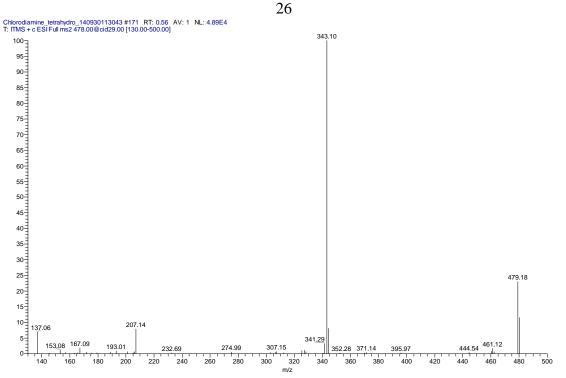
**Figure 2.4:** Mass spectrum of 4,4'-((7-chloro-3H-benzo[b][1,4-diazepine-2,4-diyl)bis(ethane-2,1-diyl))bis(2-methoxyphenol) (**17C**)
