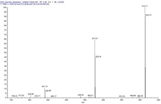
**Figure 2.10:** Mass spectrum of 4,4'-((7,8-dichloro-3H-benzo[b][1,4-diazepine-2,4-diyl)bis(ethane-2,1-diyl))bis(2-methoxyphenol) (**19**)
