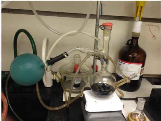
Fig 3.1: The apparatus used in the hydrogenation of curcumin
