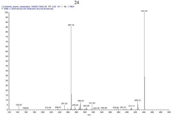
**Figure 2.3:** Mass spectrum of 4,4'-((1E,1'E)-(3H-benzo[b][1,4-diazepine-2,4-diyl)bis(ethene-2,1-diyl))bis(2-methoxyphenol) (**18b**)
