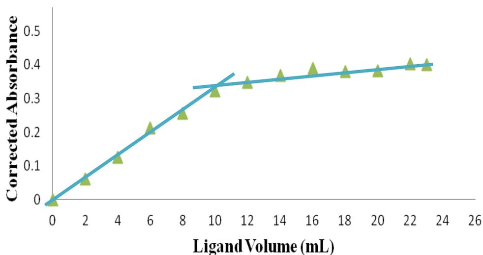
**Figure 3.16:** Spectrophotometric titration curve for the titration of  $\text{Cu}^{2+}$  -  $\text{Na}^{+}$  mixture (10 mL of 0.01 M each) with a 0.01 M TAHA. ( $\text{pH} = 10$ ,  $\lambda = 736$  nm). Absorbance was corrected by the modified correction method.
