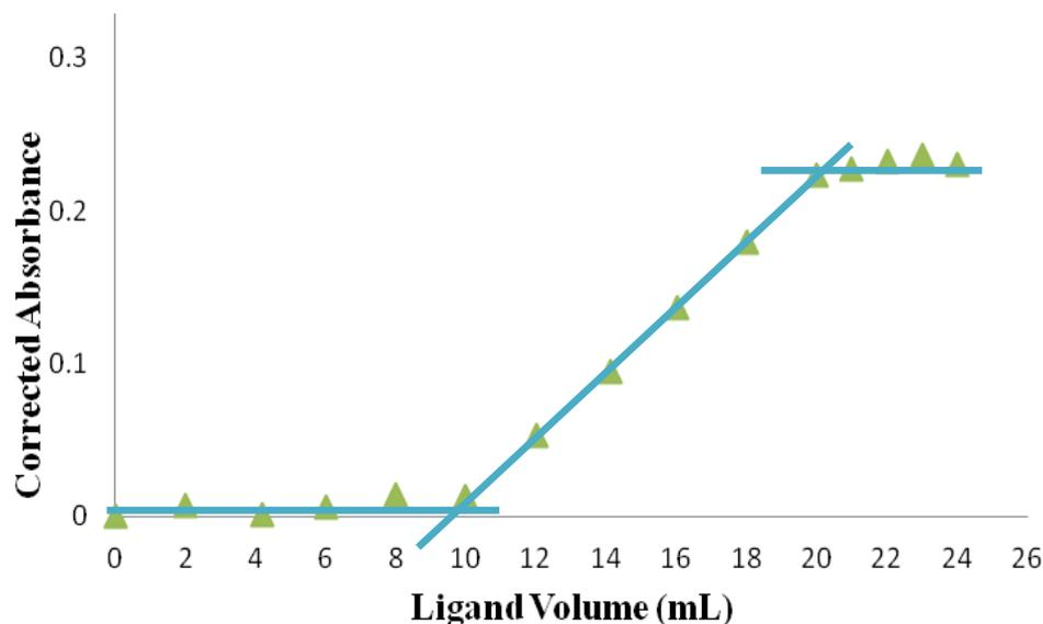
**Figure 3.14:** Spectrophotometric titration curve for the titration of  $\text{Cu}^{2+}$ -  $\text{Ca}^{2+}$  mixture (10 mL of 0.01 M each) with a 0.01 M TAHA. ( $\text{pH} = 10$ ,  $\lambda = 736$  nm). Absorbance was corrected by the modified correction method.
