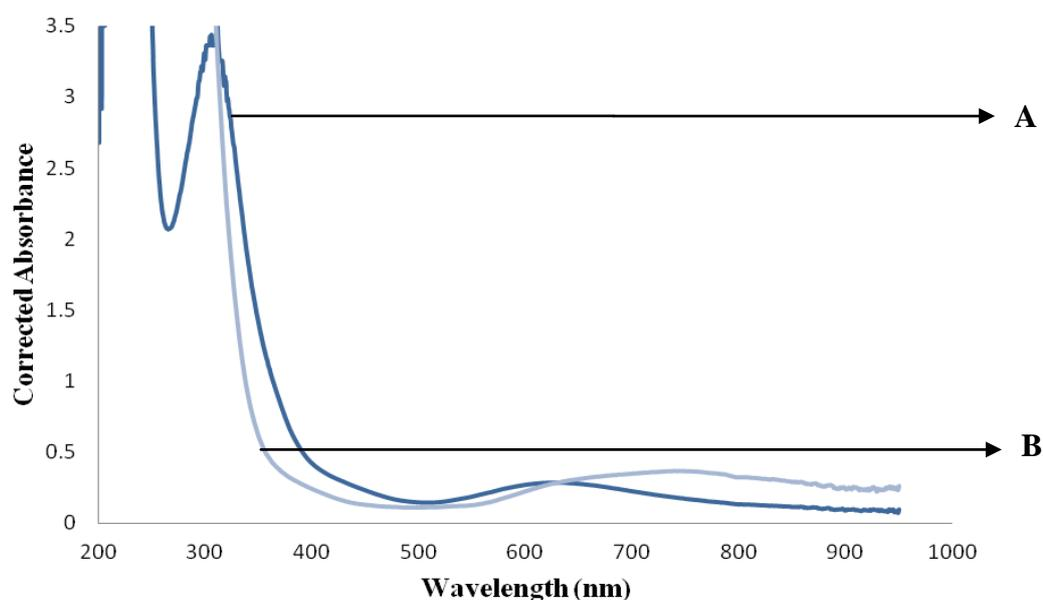
**Figure 3.17:** Absorption spectra at pH 10. A)  $\text{Cu}^{2+}$  -  $\text{Co}^{2+}$  mixture (10 mL of 0.01 M each). B) A plus 20 mL of a 0.01 M TAHA. Absorbance was corrected for dilution.
