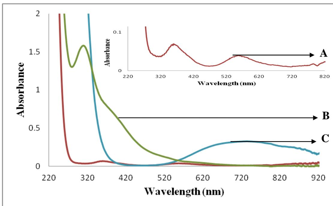
**Figure 3.6:** Absorption spectra of various M(II)-TAHA complexes at pH 10; (10 mL of 0.01 M  $M^{2+}$  plus 10 mL of 0.01 M TAHA). A)  $Ni^{2+}$ . B)  $Co^{2+}$ . C)  $Cu^{2+}$ .
