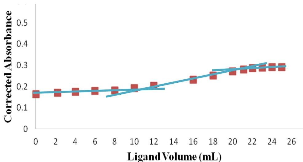
**Figure 3.21:** Spectrophotometric titration curve for the titration of  $\text{Cu}^{2+}$ - $\text{Ni}^{2+}$  mixture (10 mL of 0.01 M each) with a 0.01 M TAHA. ( $\text{pH} = 10$ ,  $\lambda = 736 \text{ nm}$ ). Absorbance was corrected for dilution.
