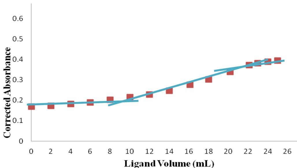
**Figure 3.23:** Spectrophotometric titration curve for the titration of  $\text{Cu}^{2+}$ -  $\text{Cd}^{2+}$  mixture (10 mL of 0.01 M each) with a 0.01 M TAHA. ( $\text{pH} = 10$ ,  $\lambda = 736$  nm). Absorbance was corrected for dilution.
