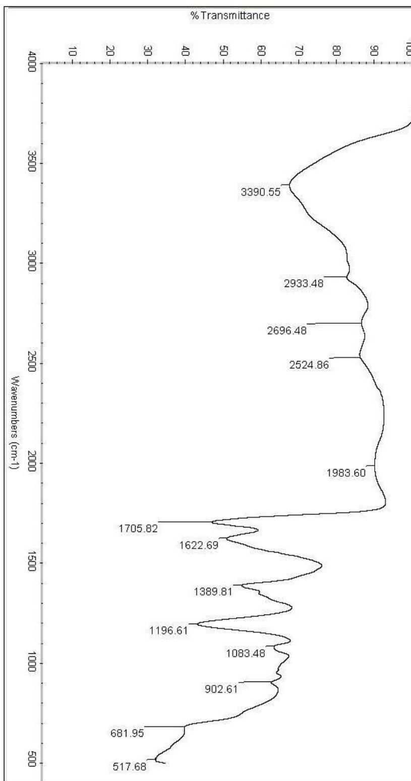
**Figure 3.3:** IR spectrum of protonated Tris(2-aminoethyl)aminehexaacetic acid.
