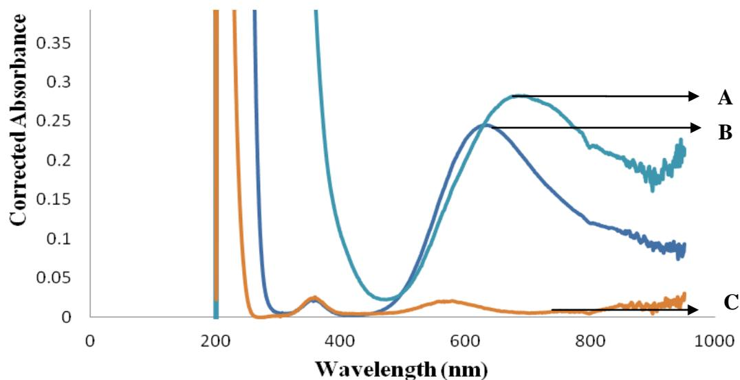
**Figure 3.20:** Absorption spectra at pH 10. A)  $\text{Cu}^{2+}$ - $\text{Ni}^{2+}$  mixture (10 mL of 0.01 M each) plus 20 mL of a 0.01 M TAHA. B)  $\text{Cu}^{2+}$ - $\text{Ni}^{2+}$  mixture (10 mL of 0.01 M each). C)  $\text{Ni}^{2+}$  (10 mL of 0.01M). Absorbance was corrected for dilution.
