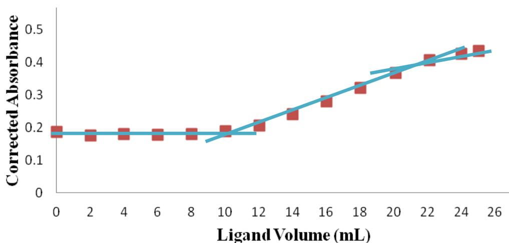
**Figure 3.18:** Spectrophotometric titration curve for the titration of  $\text{Cu}^{2+}$  -  $\text{Co}^{2+}$  mixture (10 mL of 0.01 M each) with a 0.01 M TAHA. (pH = 10,  $\lambda = 736$  nm). Absorbance was corrected for dilution.
