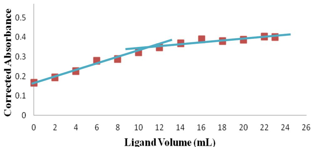
**Figure 3.15:** Spectrophotometric titration curve for the titration of  $\text{Cu}^{2+}$  -  $\text{Na}^{+}$  mixture (10 mL of 0.01 M each) with a 0.01 M TAHA. ( $\text{pH} = 10$ ,  $\lambda = 736$  nm). Absorbance was corrected for dilution.
