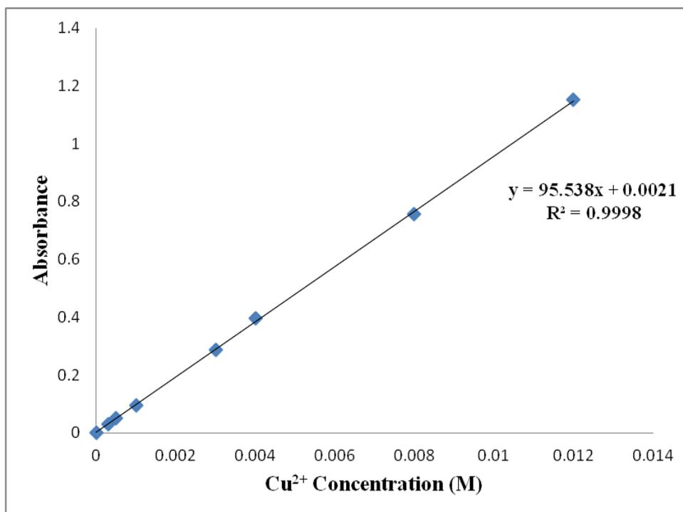
**Figure 3.27:** Calibration curve for Cu(II) at pH 10,  $\lambda = 736$  nm.
