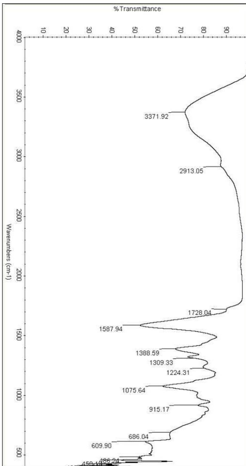
**Figure 3.4-a:** IR spectra of Copper(II)-TAHA complex (4000- 500 cm<sup>-1</sup>)
