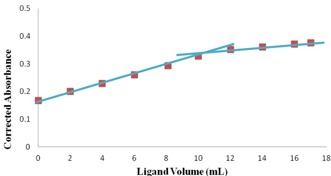
**Figure 3.7:** Spectrophotometric titration curve for the titration of 10 mL of 0.01 M  $\text{Cu}^{2+}$  with a 0.01 M TAHA. (pH = 10,  $\lambda = 736$  nm).
