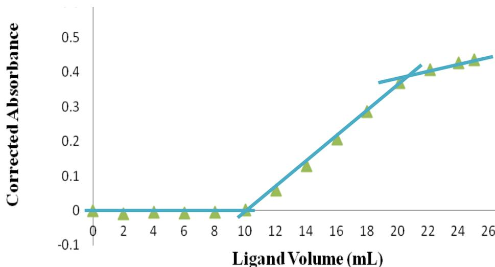
**Figure 3.19:** Spectrophotometric titration curve for the titration of  $\text{Cu}^{2+}$ -  $\text{Co}^{2+}$  mixture (10 mL of 0.01 M each) with a 0.01 M TAHA. ( $\text{pH} = 10$ ,  $\lambda = 736 \text{ nm}$ ). Absorbance was corrected by the modified correction method.
