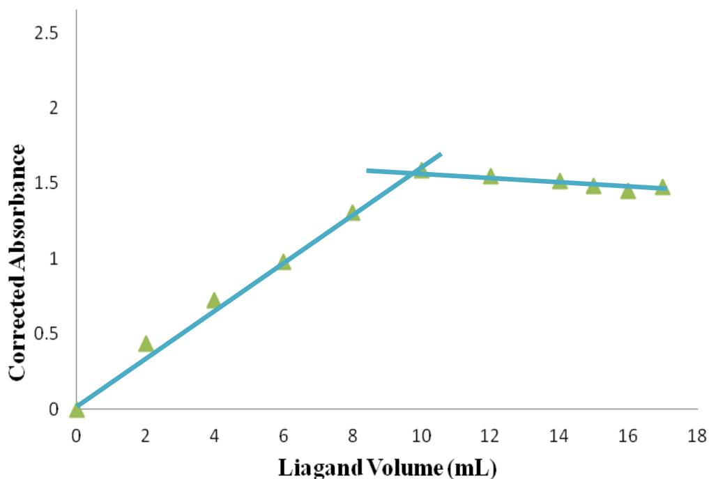
**Figure 3.10:** Spectrophotometric titration curve for the titration of 10 mL of 0.01 M  $\text{Co}^{2+}$  with a 0.01 M TAHA. (pH = 10,  $\lambda = 309$  nm). Absorbance was corrected by the modified correction method.
