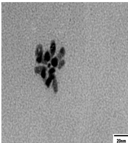
Fig 3.39: The TEM image of TOAB stabilized S NPs prepared at 60°C using (2 M HCl).
