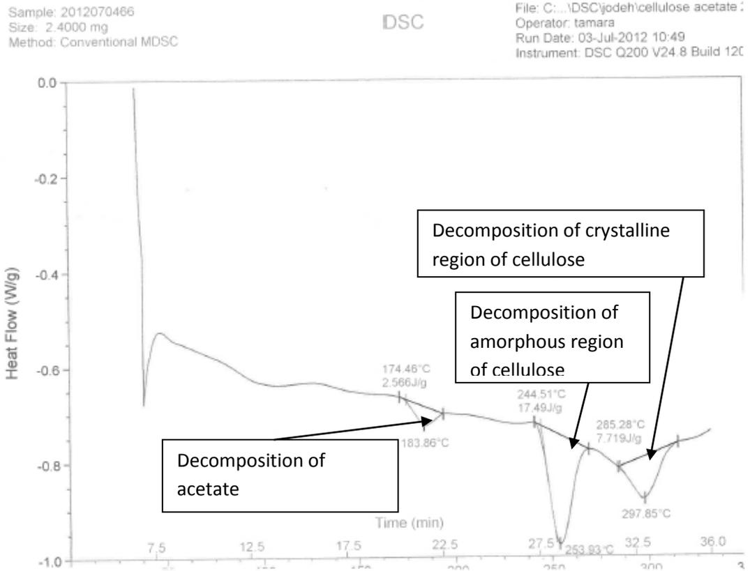
**Figure 3.26:** DSC of cellulose acetate made under heterogeneous conditions
