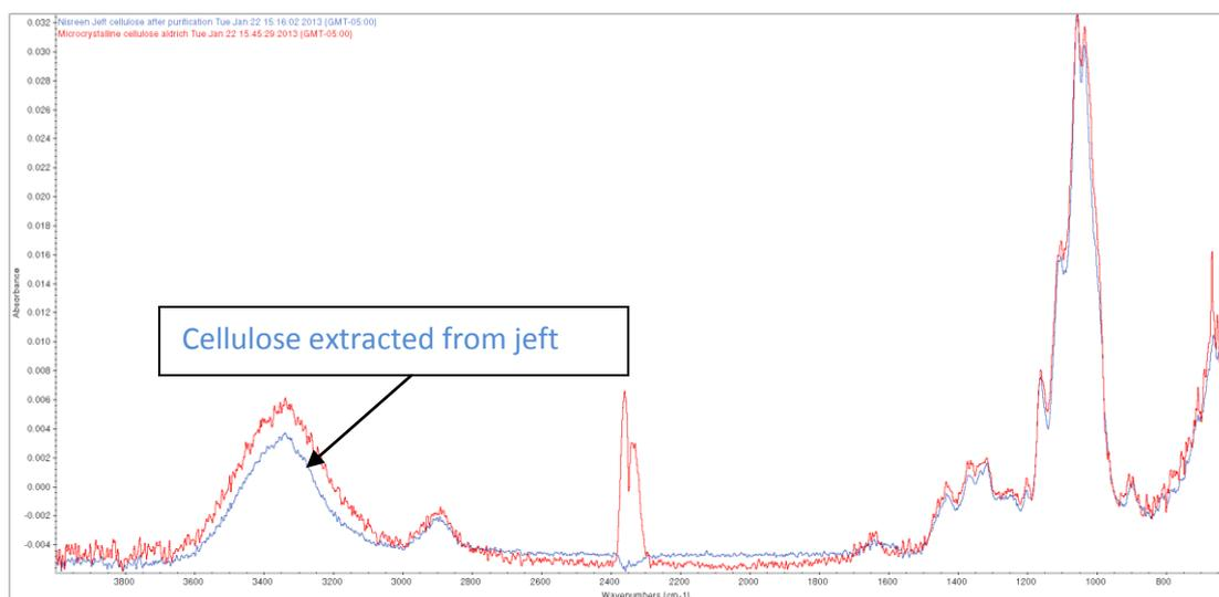
**Figure 3.8:** IR spectra of cellulose extracted from jeft and microcrystalline cellulose
