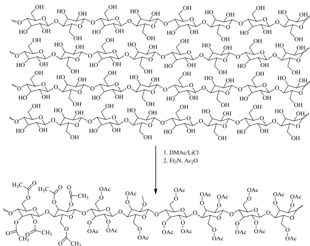
**Figure 3.12:** Converting cellulose into cellulose acetate
