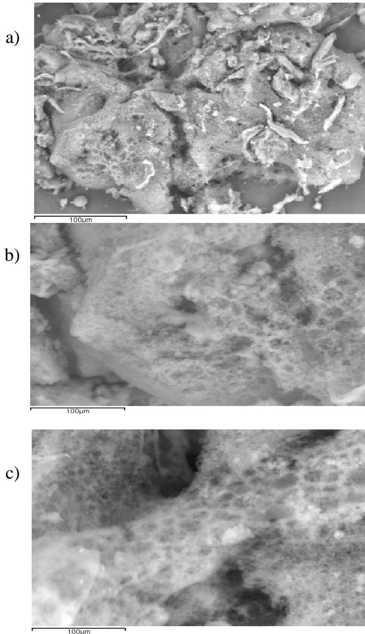
**Figure 3.15:** SEM images of cellulose acetate at three different magnifications; a) 300x, b) 500x, and c) 1000x
