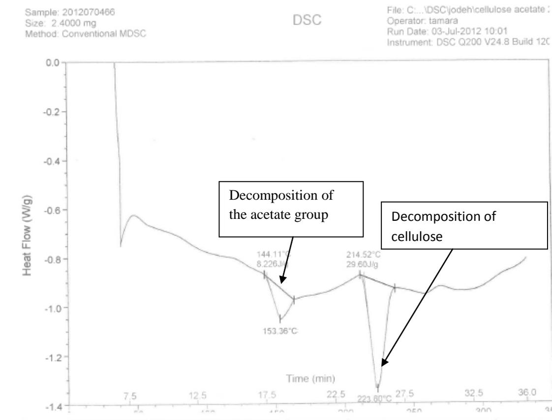
**Figure 3.20:** DSC of cellulose acetate made under homogeneous conditions
