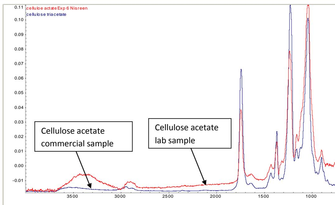
**Figure 3.22:** IR spectra of cellulose acetate prepared under heterogeneous conditions
