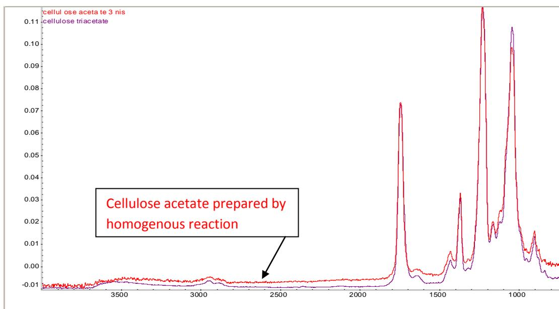
**Figure 2.2** FTIR results for cellulose acetate prepared by homogeneous method
