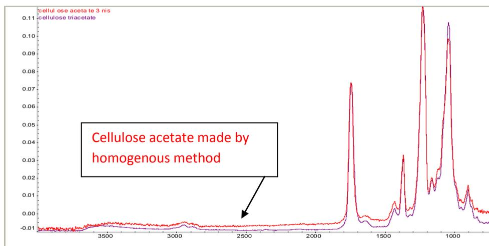
**Figure 3.14:** IR spectra of cellulose acetate made from cellulose extracted from jeft and cellulose acetate obtained from Aldrich Chemical Company
