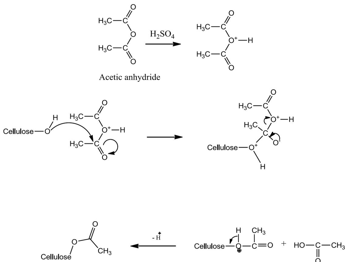
**Figure 3.21:** Reaction mechanism for acetylation of cellulose under heterogeneous conditions:
