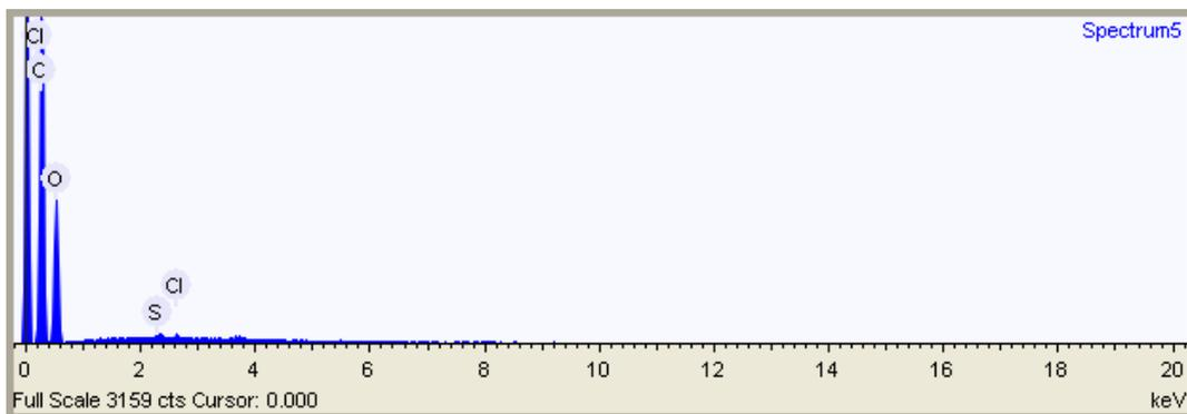
**Figure 3.17:** X-ray of cellulose acetate prepared by homogeneous method-Run 2
