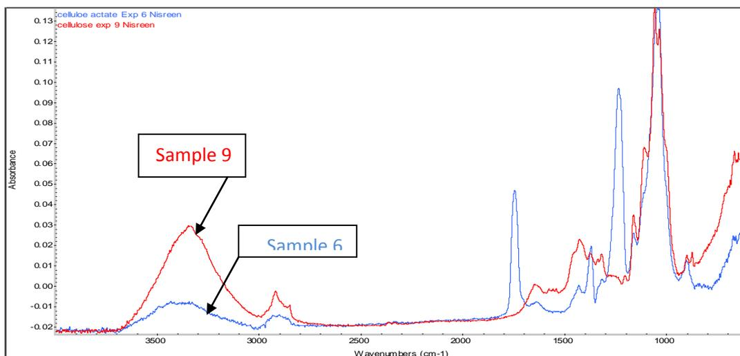
**Figure 2.1: FTIR results for cellulose acetate samples number 6 and 9**
