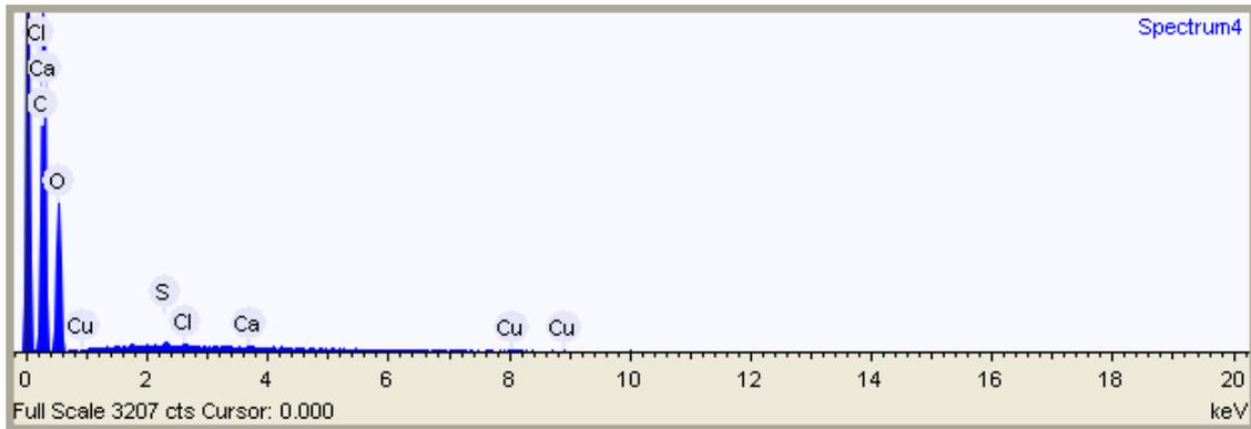
**Figure 3.16 :** X-ray of cellulose acetate prepared by homogeneous method-Run 1
