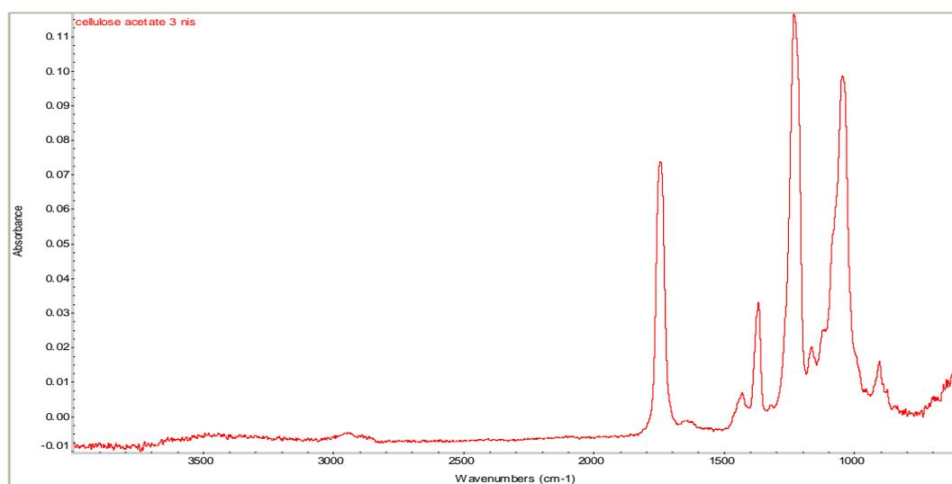
**Figure 3.13:** IR spectra of cellulose acetate prepared from cellulose extracted from jeft.
