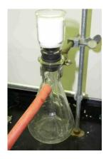
Figure 1.5: Dry column flash chromatography setup
