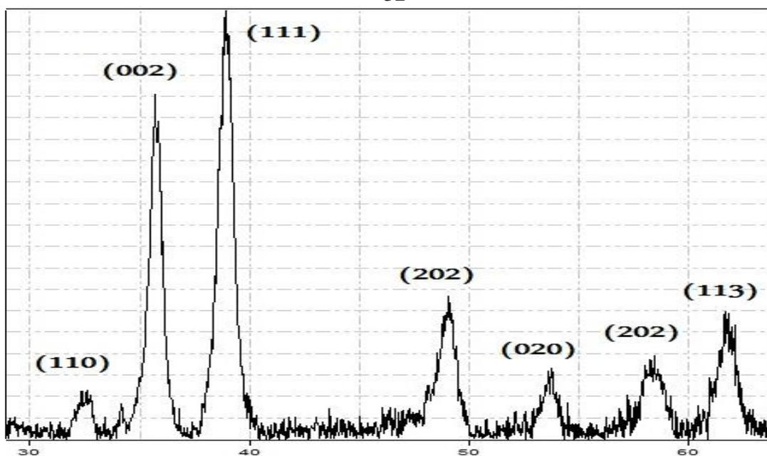
**Fig 3.1:** XRD pattern of CuO nanoparticles were prepared at 65 °C with TOAB surfactant.
