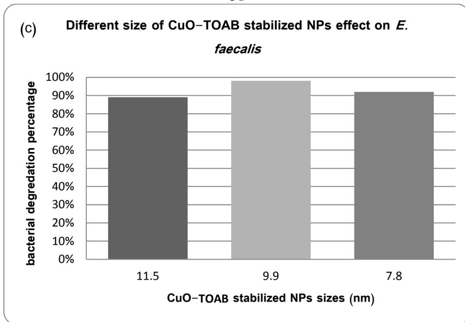
**Fig. 3.15:** CuO NPs size with surfactant effect on a) TC b) FC and c) *E. faecalis*.
