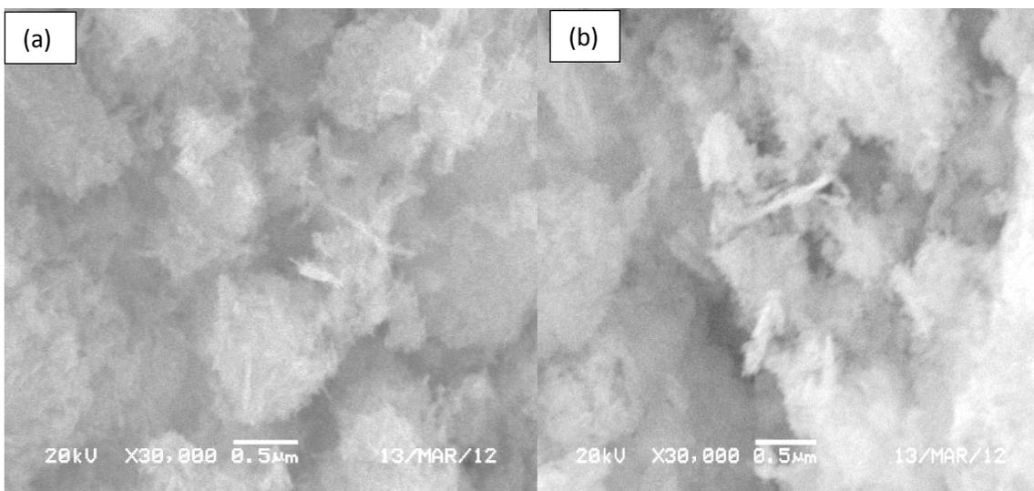
**Fig 3.9: The SEM images of CuO nanoparticles prepared at 85 °C a) with TOAB surfactant b) without TOAB surfactant**
