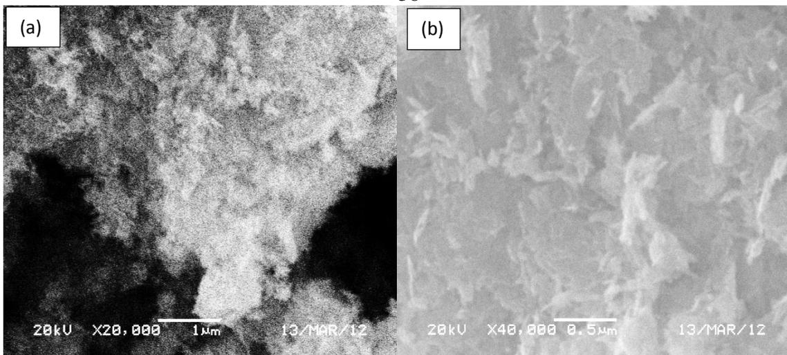
**Fig 3.8: The SEM images of CuO nanoparticles prepared at 75 °C a) with TOAB surfactant b) without TOAB surfactant.**
