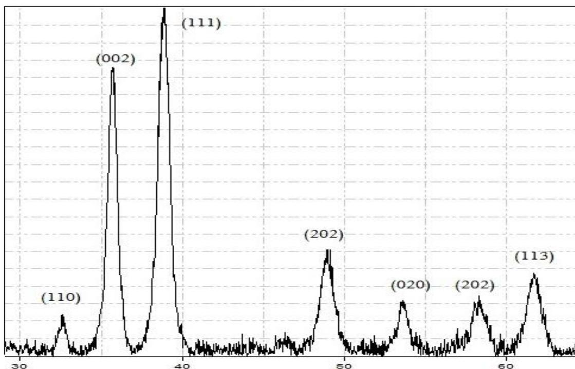
**Fig 3.3:** XRD pattern of CuO nanoparticles were prepared at 75 °C with TOAB surfactant
