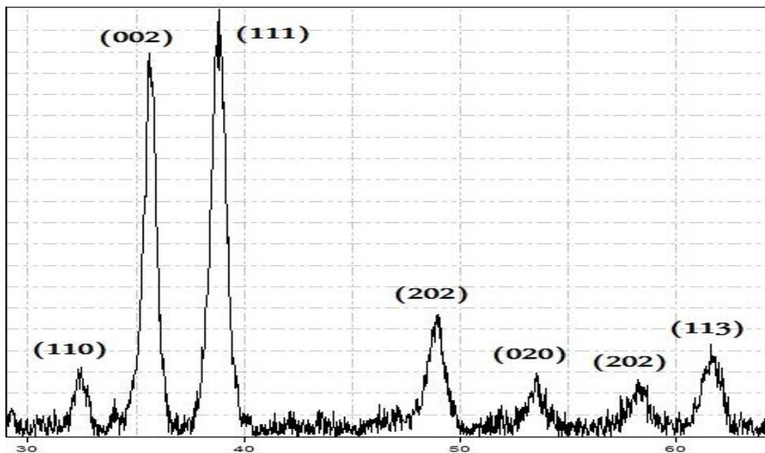
**Fig 3.2:** XRD pattern of CuO nanoparticles were prepared at 65 °C without TOAB surfactant
