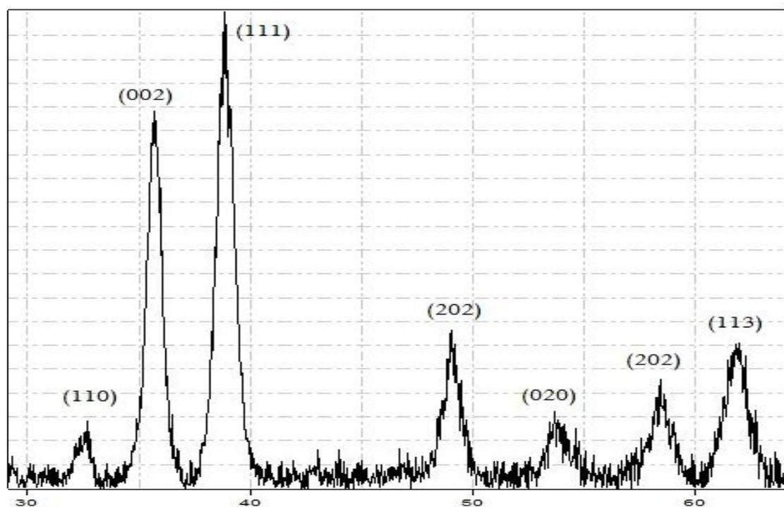
**Fig 3.4:** XRD pattern of CuO nanoparticles were prepared at 75 °C without TOAB surfactant
