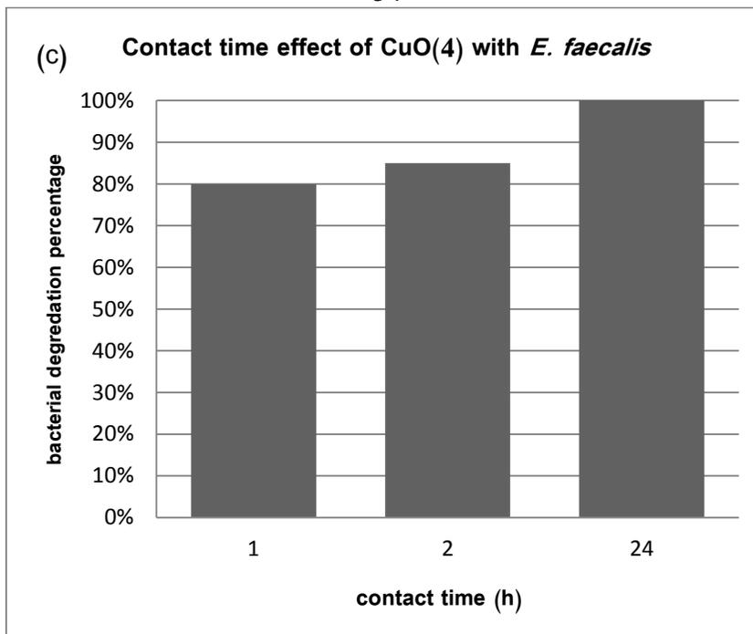
Fig 3.16: 1, 2 and 24 h contact time effect of CuO(4) on a) TC b) FC c) *E. faecalis*
