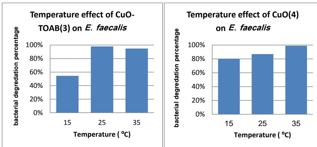
**Fig 3.20: The effect of wastewater temperature (15, 25 and 35 °C) on degradation percentage of *E. faecalis* using a) CuO-TOAB(3) and b) CuO(4)**
