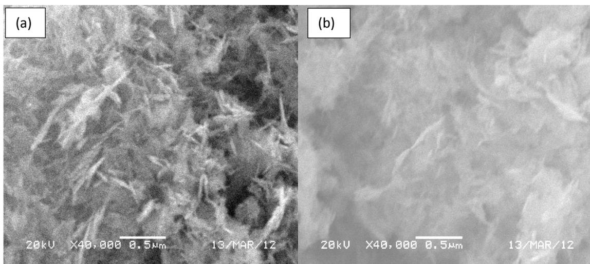
**Fig 3.7: The SEM images of CuO nanoparticles prepared at  $65^\circ\text{C}$  a) with TOAB surfactant b) without TOAB surfactant.**
