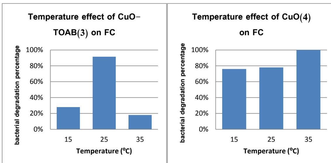
**Fig 3.19: The effect of wastewater temperature (15, 25 and 35 °C) on degradation percentage of FC using a) CuO-TOAB(3) and b) CuO(4)**
