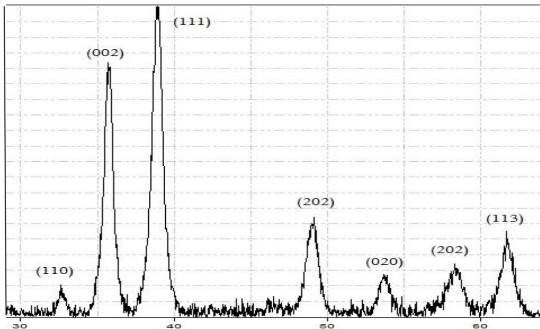
**Fig 3.6: XRD pattern of CuO nanoparticles were prepared at 85 °C without TOAB surfactant**
