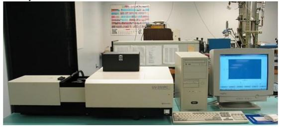
Fig (3.2): UV-Visible spectrophotometer
