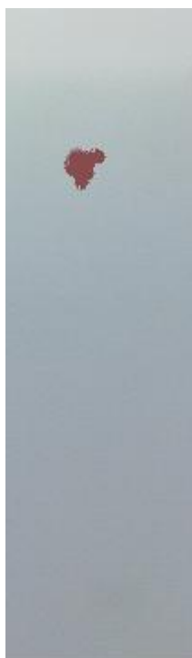
Figure 3.6: TLC measured for one anthocyanin solution, showing only one component for extracted dyes.
