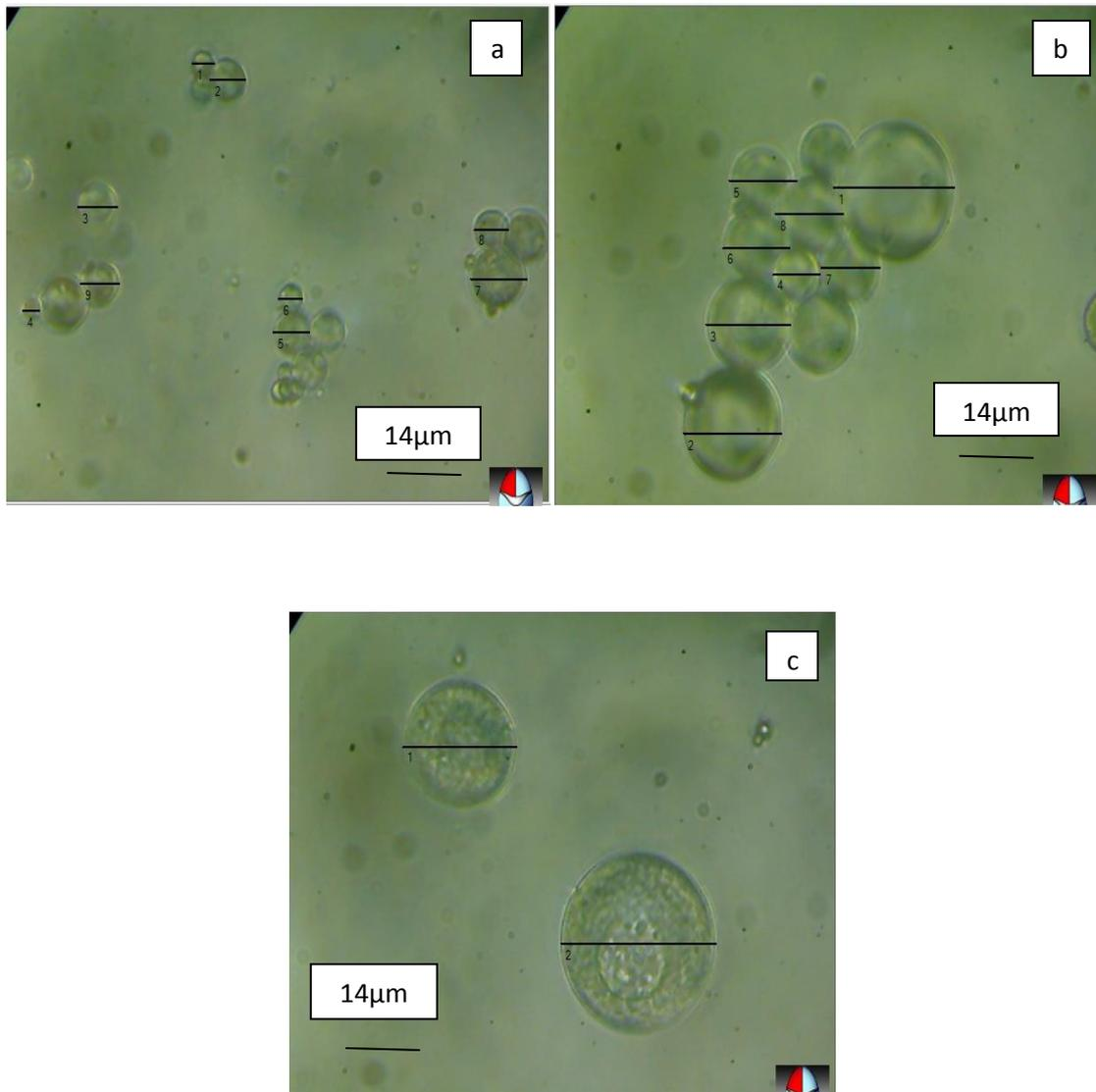
**Figure 3. 1.** The size of PLG microcapsules prepared with a) 10% (w/w) SDS solution, b) 5% (w/w) SDS solution and c) 2% (w/w) SDS solution, measured by light microscope.
