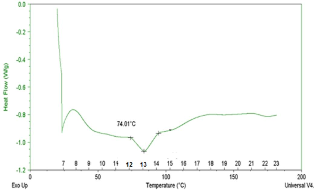
**Figure 3.8.** DSC result for PLG microcapsules prepared with 18% methanol.
