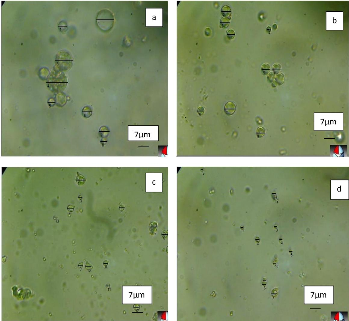
**Figure 3. 3** : The size of PLG microcapsules prepared with (10 % (w/w) SDS solution) and a) 9% methanol b) 18% methanol c) 27% methanol d) 18% ethanol, measured by light microscope.
