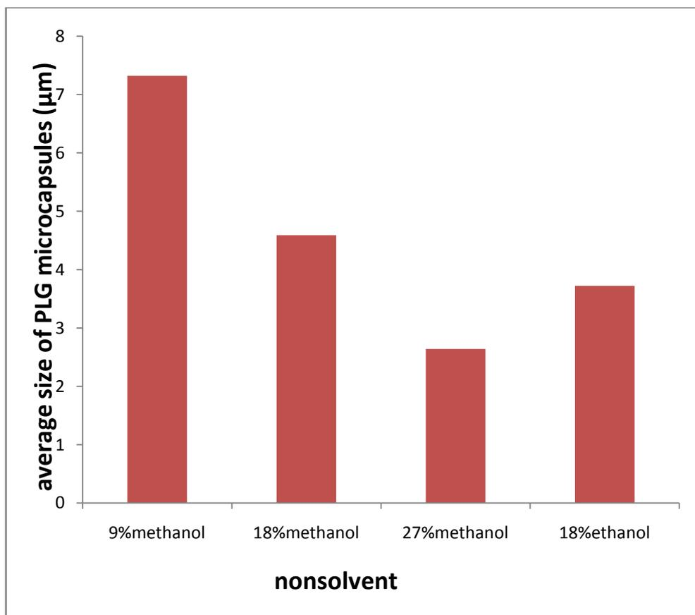
**Figure 3 .4: (a):** The average size of PLG microcapsules prepared with different concentration of methanol and ethanol.
