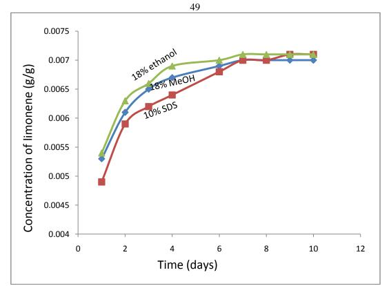
Figure 3.14. Limonene release from PLG microcapsules prepared with amount of methanol, ethanol solutions
