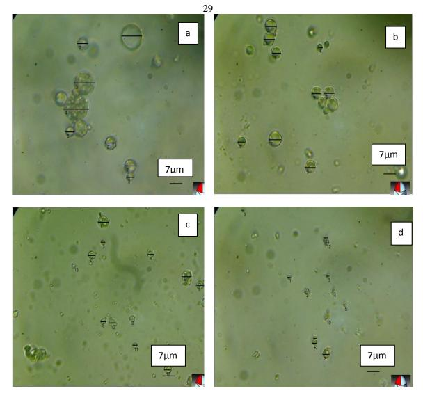
Figure 3. 3 : The size of PLG microcapsules prepared with (10 % (w/w) SDS solution) and a) 9% methanol b) 18% methanol c) 27% methanol d) 18% ethanol, measured by light microscope.
