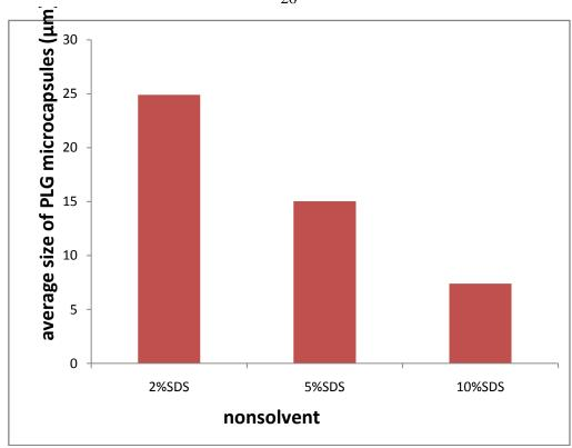
Figure 3.2: (a): The average size of PLG microcapsules prepared with different concentration of SDS solution.
