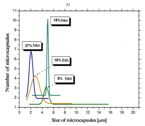
Figure 3. 4 (b): The size distribution of PLG microcapsules prepared with different concentration of methanol and ethanol.
