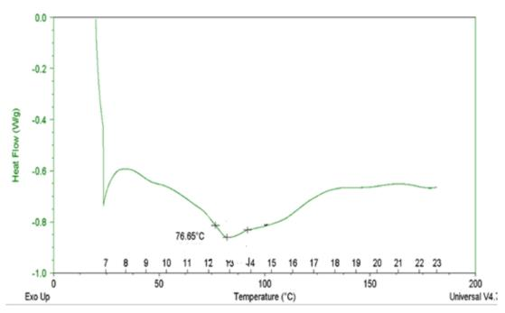
Figure 3.9: DSC result for PLG microcapsules prepares with 27% methanol.
