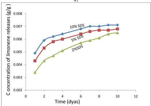
**Figure 3.12**: limonene release from PLG microcapsules prepared with different amount of SDS solution.
