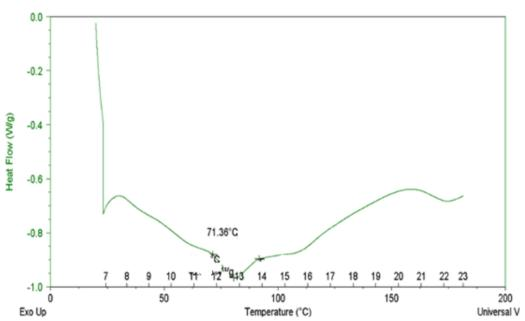
Figure 3.7. DSC result for PLG microcapsules prepares with 2% SDS solution.
