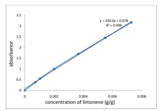
**Figure 3.11:** A typical calibration curve for limonene in 0 .1M potassium phosphate buffer analysis by UV-VIS spectrometric method.
