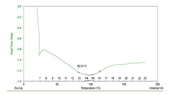
Figure 3.10: DSC result for PLG microcapsules prepares with 18% ethanol.
