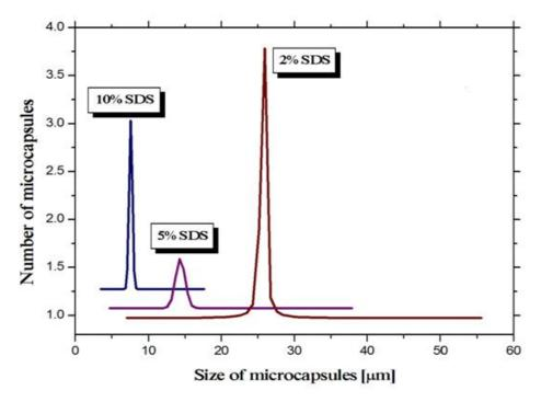
Figure 3.2: (b): The size distribution of PLG microcapsules prepared with different concentration of SDS solution.
