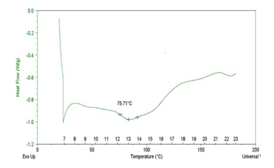
Figure 3.6. DSC result for PLG microcapsules prepares with 10% SDS solution.
