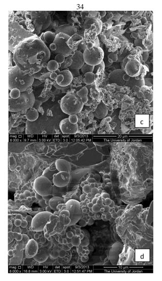
Figure 3.5: SEM micrographs of prepared microcapsules with a) 10% SDS, b) 5% SDS, c) 18% methanol, d) 18% ethanol.
