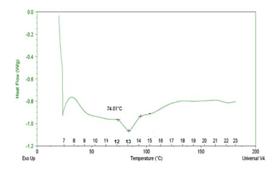
Figure 3.8. DSC result for PLG microcapsules prepares with 18% methanol.
