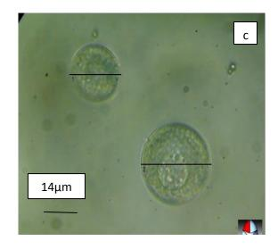
**Figure 3. 1.** The size of PLG microcapsules prepared with a) 10% (w/w) SDS solution, b) 5% (w/w) SDS solution and c) 2% (w/w) SDS solution, measured by light microscope.
