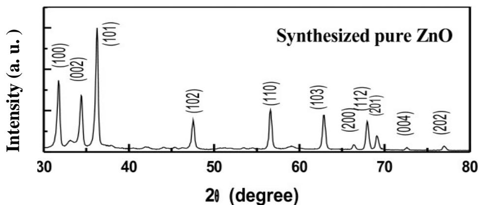
**Figure (1.2):** XRD pattern for ZnO nanoparticles [62].
