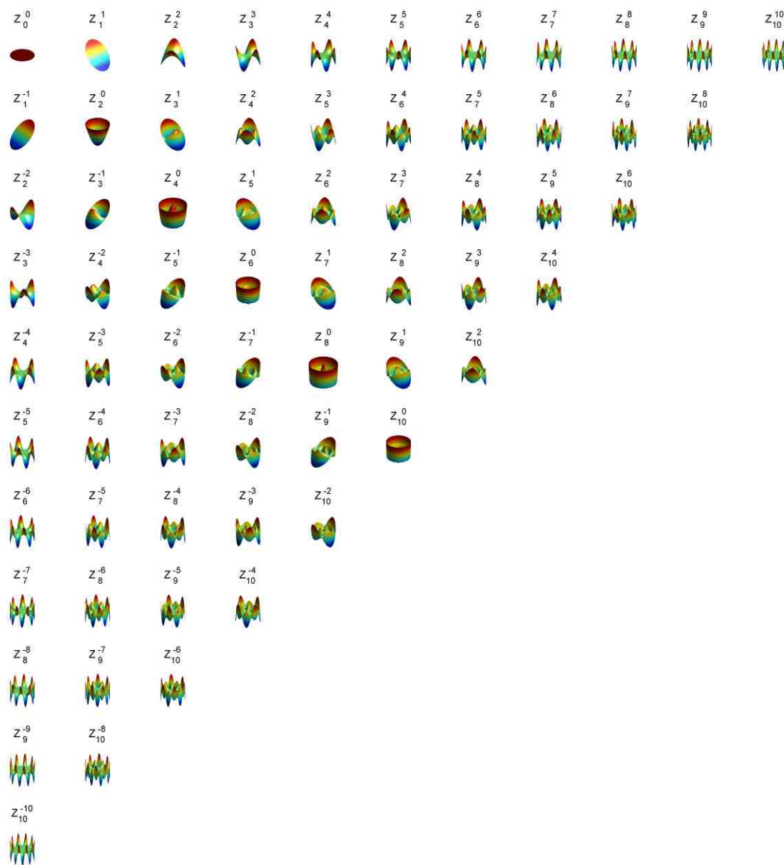
Figure 2.2: The continuous Zernike polynomials plotted in 3 dimensions up to the 10 th degree.
