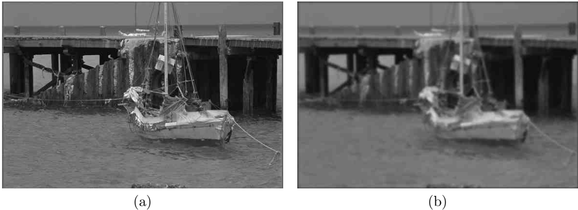
Figure 3.30: An original image in grayscale (a), and the smoothed version in (b) using a Gaussian, low-pass filter with standard deviation of 4 pixels (1.6% of \rho_0 ).
