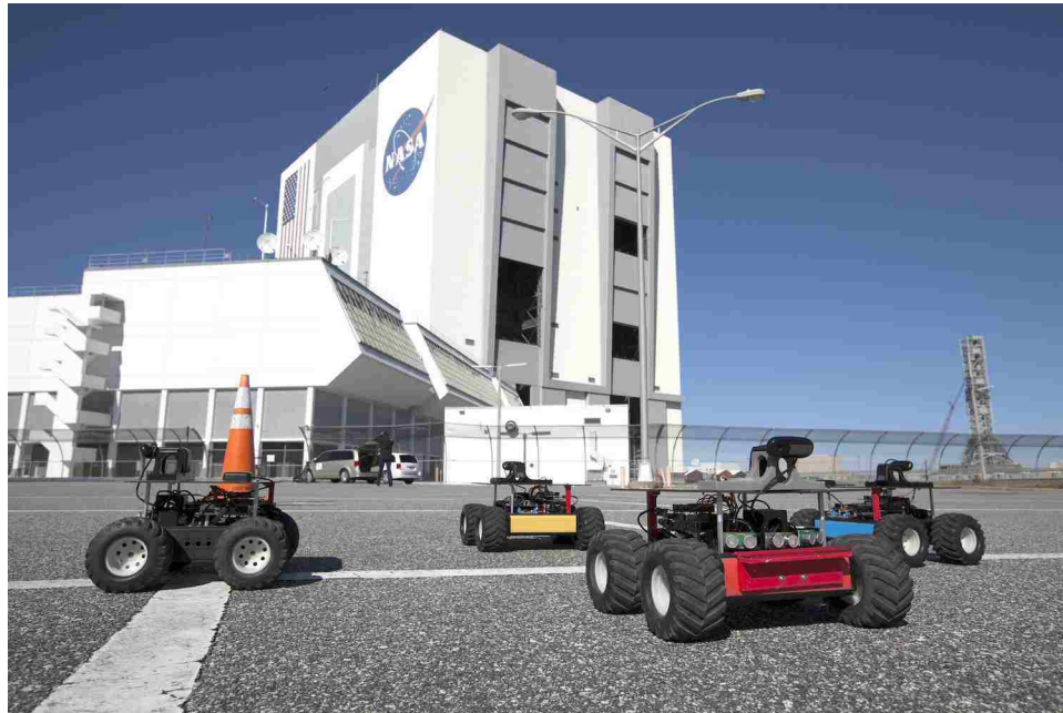
Figure 6.1: The Swarmie hardware platform developed through a UNM partnership with NASA Kennedy Space Center’s (KSC) Swamp Works laboratory. The Swarmie platform is an integrated system with adaptive software and a simulator that allows rapid testing of new algorithms in software and rapid porting to hardware for verification in physical experiments.
