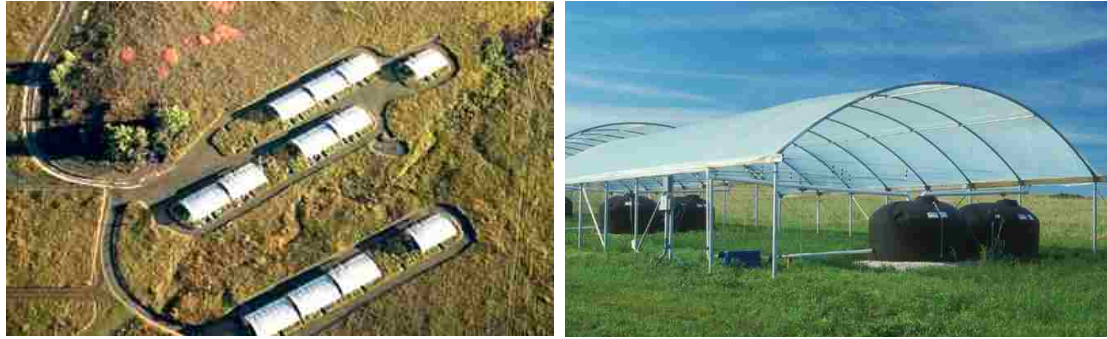
Figure 2. a) Aerial overview of Rainfall Manipulation Plots (RaMPs) layout and b) a side view of a RaMP showing watering tanks.
