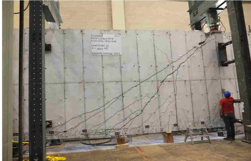
Figure 6.16 – Shear failure in west side of Toronto beam at 2162 kN (486 kips)
