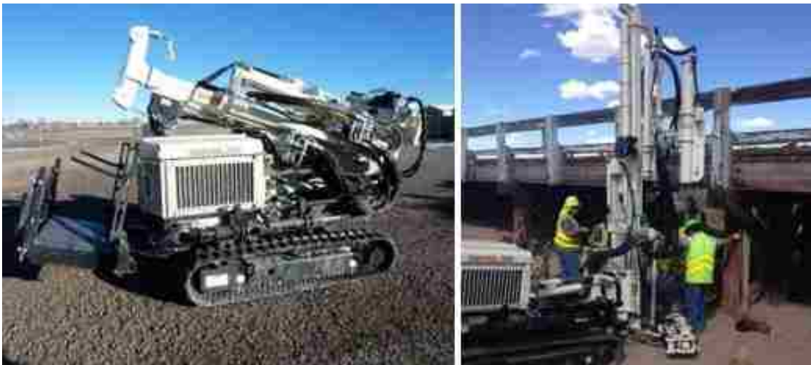
Figure 163. Geoprobe Model 7822DT- Low Headroom Drill Rig
