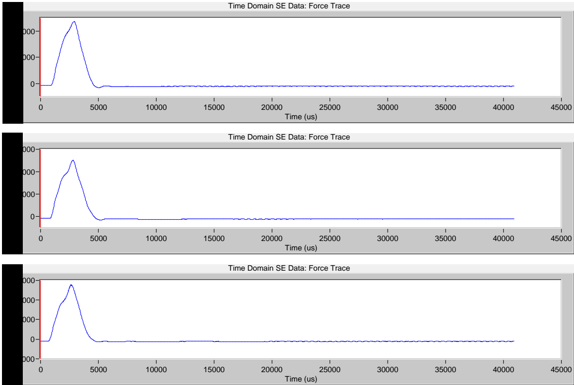
Figure 82. Initial Hammer Impulses (Wooden blocks, Medium-hard-tip)
