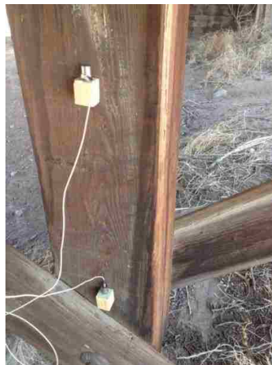
Figure 118. Accelerometers Attached onto a Pile
