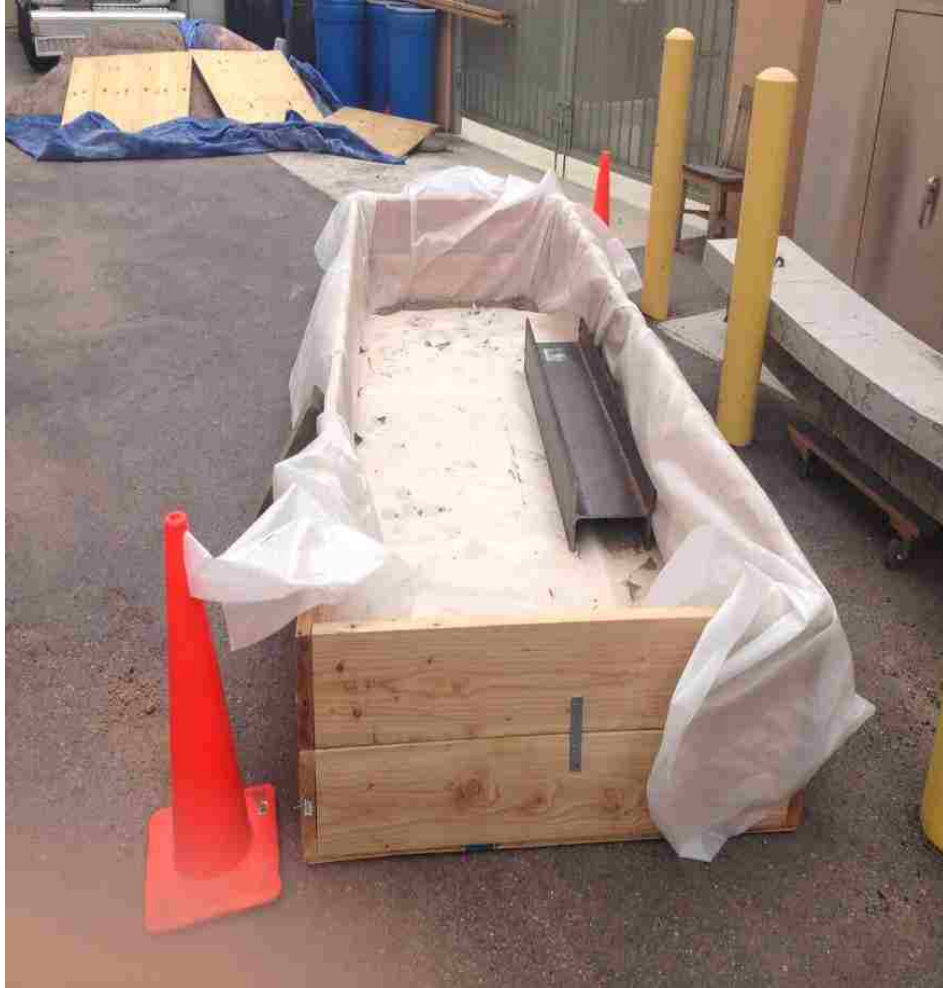
Figure 180. Test Configuration with Steel Beam and Wooden Box
