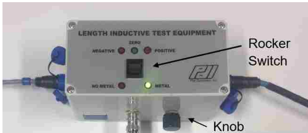
Figure 178. Details of Signal Conditioning Box
