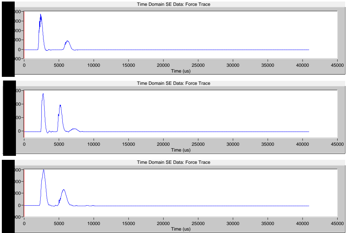
Figure 86. Impulse Signals Generated by Striking the Aluminum Block with Hard Hammer Tips (Tests 17 to 19)
