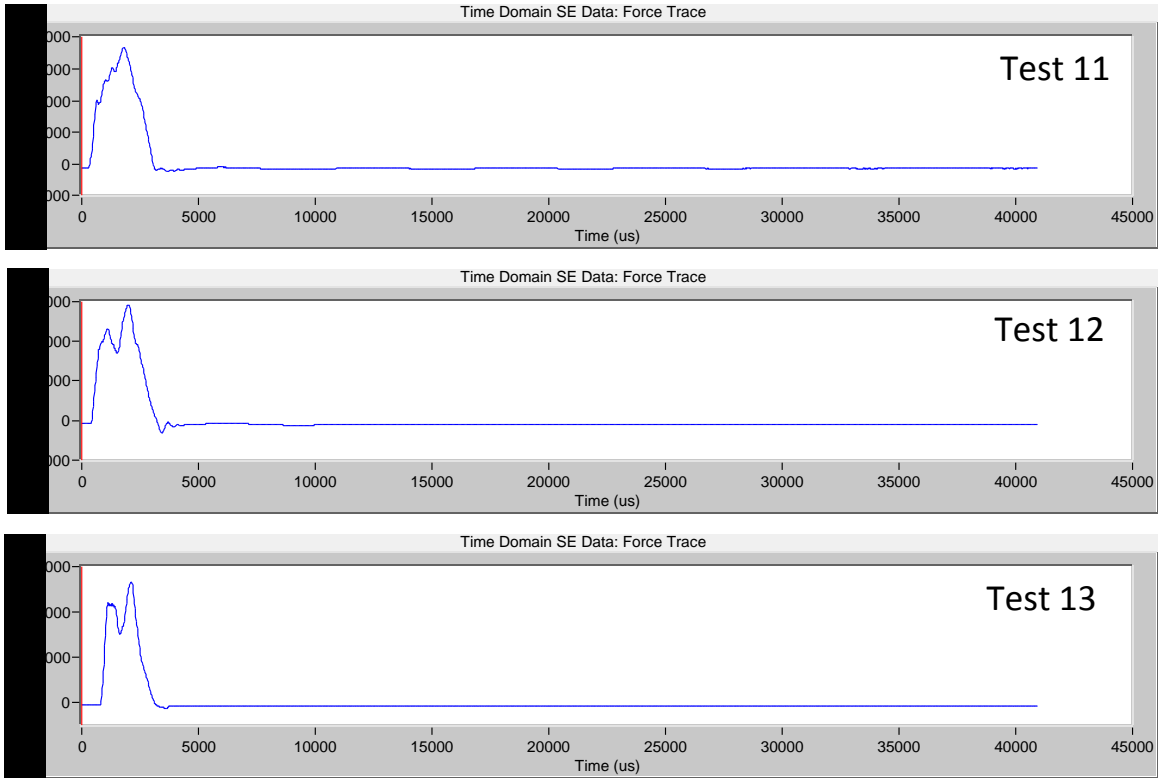
Figure 78. Initial Impulse from the Hammer's Force Sensor (Wooden block, Hard-tip)
