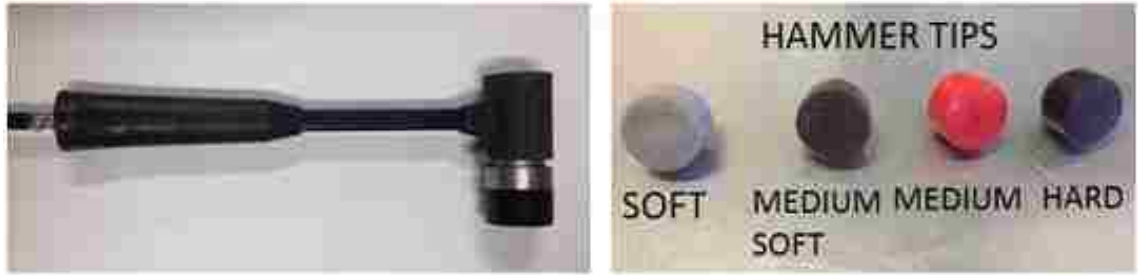
Figure 28. A Hammer and Four Different Tips
