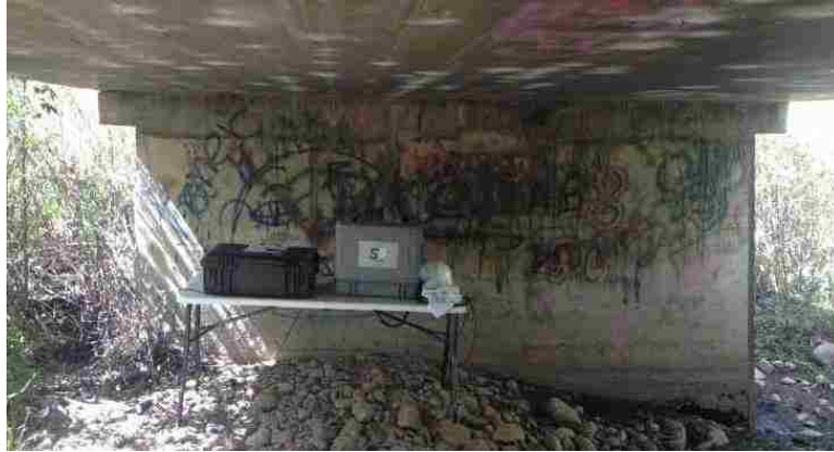
Figure A22. SE/IR Equipment Placement near a Test Pier Wall
