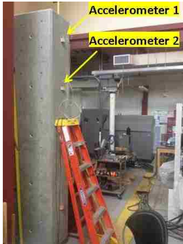
Figure 45. An SE Setup on the Reinforced Concrete Wall
