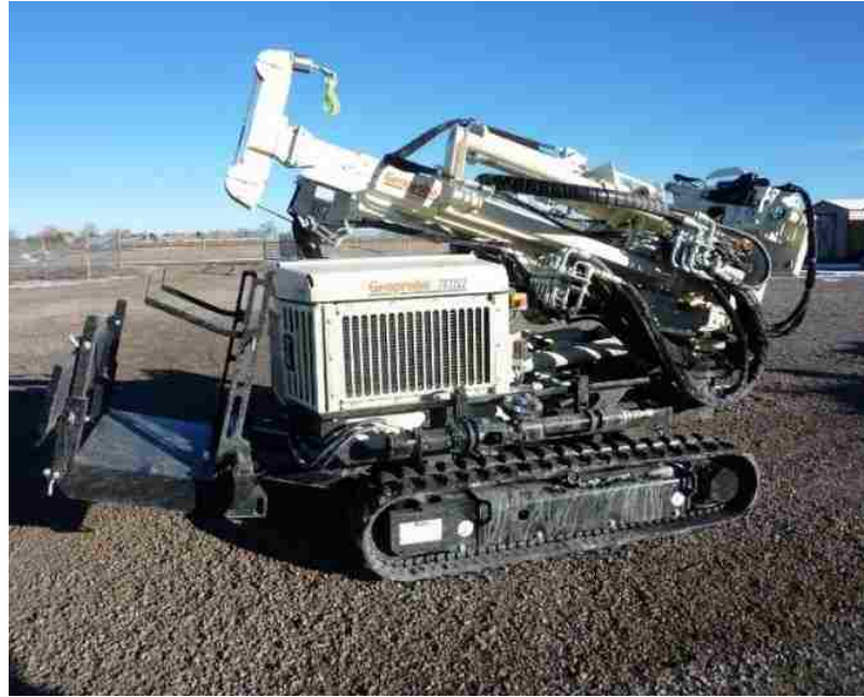
Figure A1. Geoprobe 7822DT-Low Headroom Drill Rig
