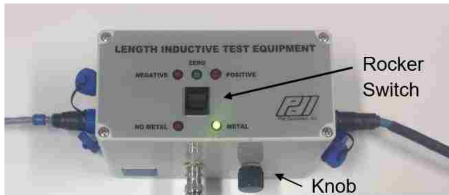
Figure A48. Details of Signal Conditioning Box
