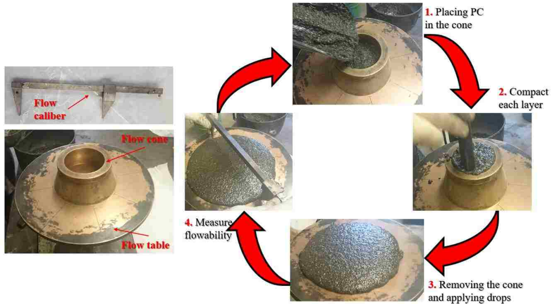
Figure 3.4: Flowability measurement of PC showing flow caliber, cone and table and test procedure.
