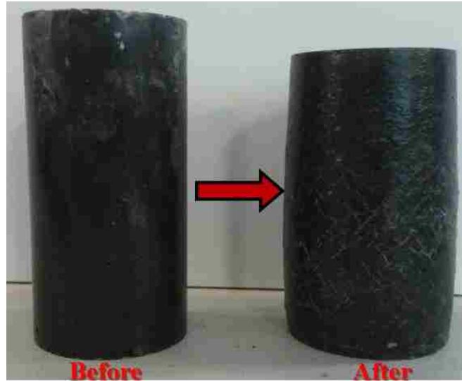
Figure 4.57: Before and after compression test showing extreme ductility of NPC-Neat
