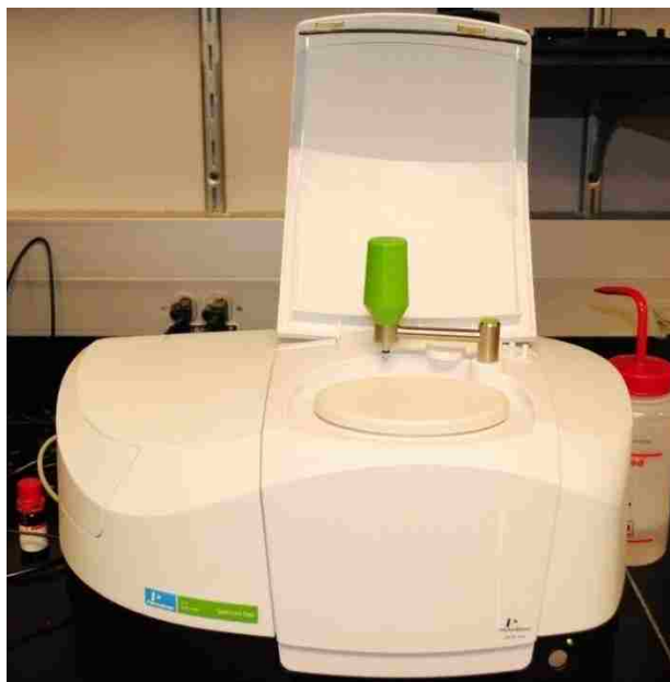
Figure 3.23: PerkinElmer FTIR machine used in microstructural analysis.
