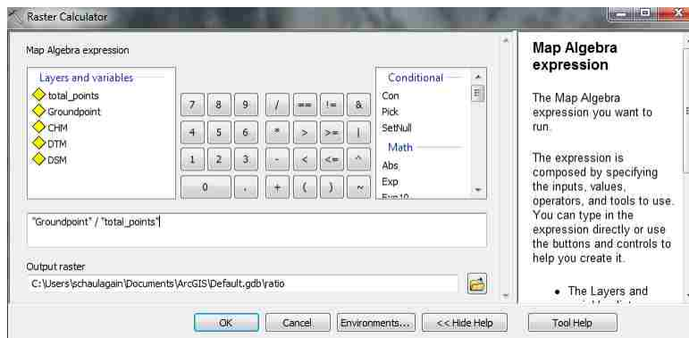
Figure 33: Raster calculator to calculate ratio of grounds to total points
