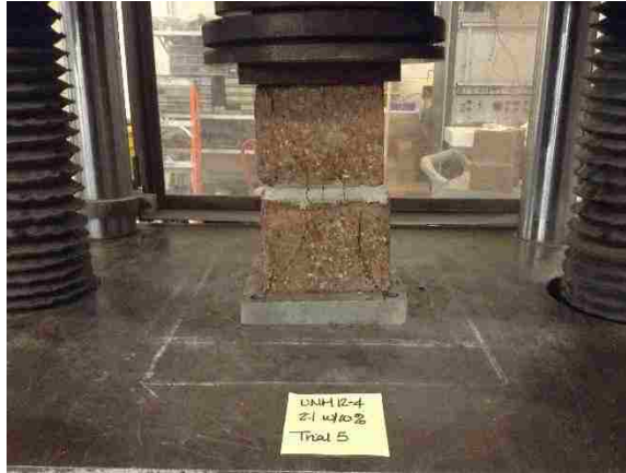
Figure 3. 34. SCEB 7 prism compression on Tinius Olsen machine.
