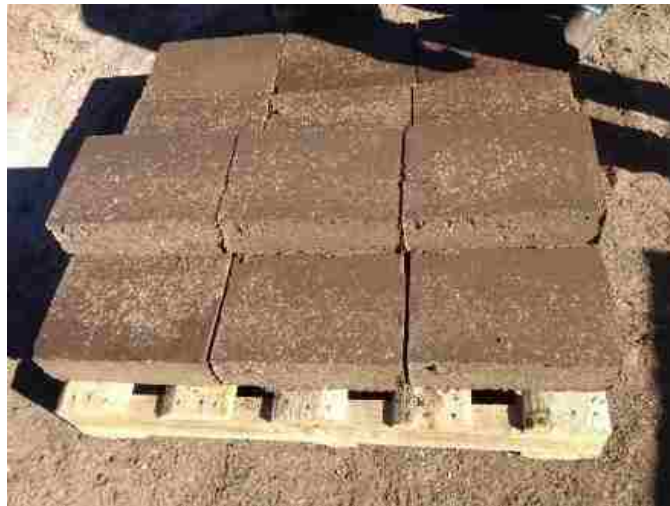
Figure 3. 18 Recently compressed SCEBs on pallet to be wrapped in order to cure.
