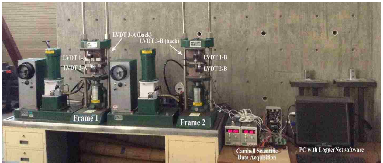
Figure 3. 35. SCEB 7 prisms placed on the Carver Press and displacement measured using the Campbell Scientific Data Acquisition.
