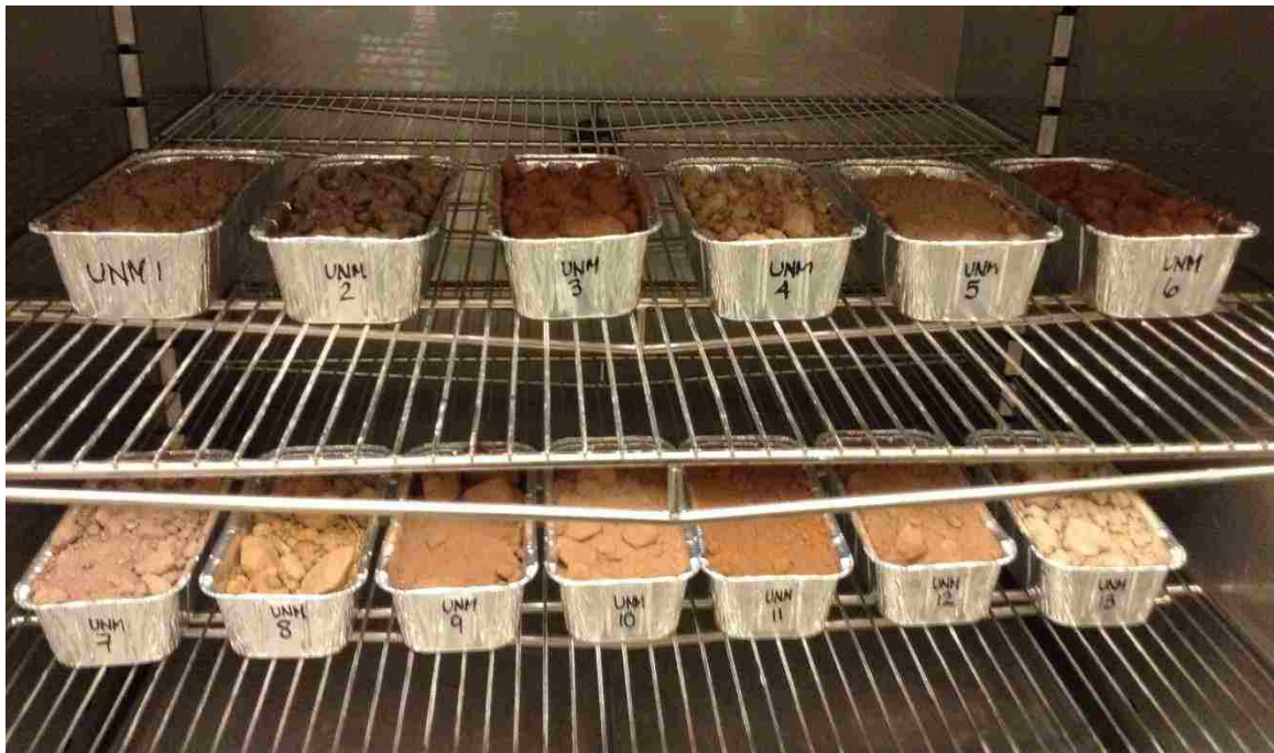
Figure 3. 6. Soil samples determining moisture content in oven at 110°C.
