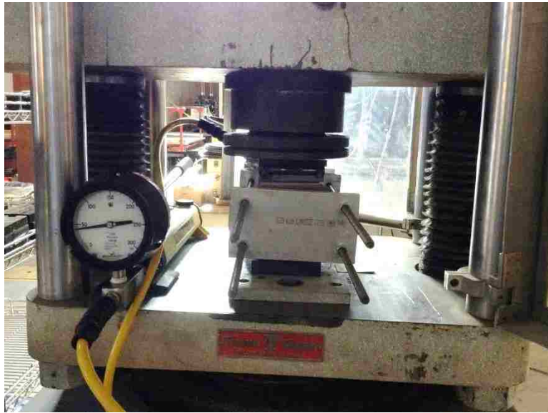
Figure 3. 41. Shear testing apparatus in the Tinius Olsen machine.
