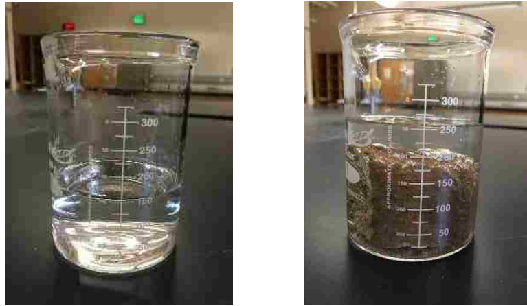
Figure 3. 28. (a) 400 mL beaker filled with 150 mL distilled water. (b) Specimen placed in 400 mL beaker.
