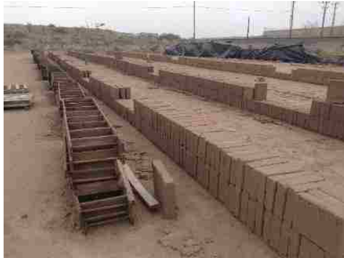
Figure 3. 19. NM Earth Adobe yard with Stabilized Adobe and Formwork shown.
