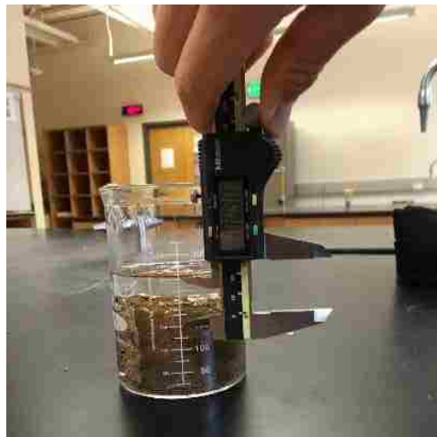
Figure 3. 29. Measuring the vertical displacement of the water level once the specimen is placed in the beaker.
