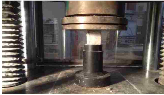
Figure 3. 33. 50mm cube specimen tested for mortar compression on the Tinius Olsen Machine.
