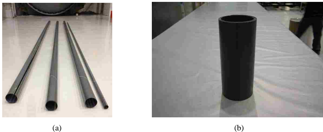
Figure 3.2: CFRP slit tube tape springs with a 101.6 mm diameter in the Integrated Structural Systems' Composites Laboratory at AFRL shown in their (a) deployed configuration and (b) stowed configuration. Images courtesy of Michael Peterson.
