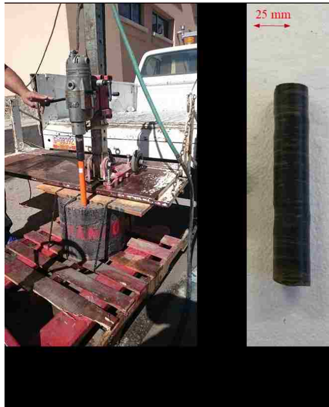
Figure 3.1: (a) Coring process of Mancos shale and (b) Mancos shale core.
