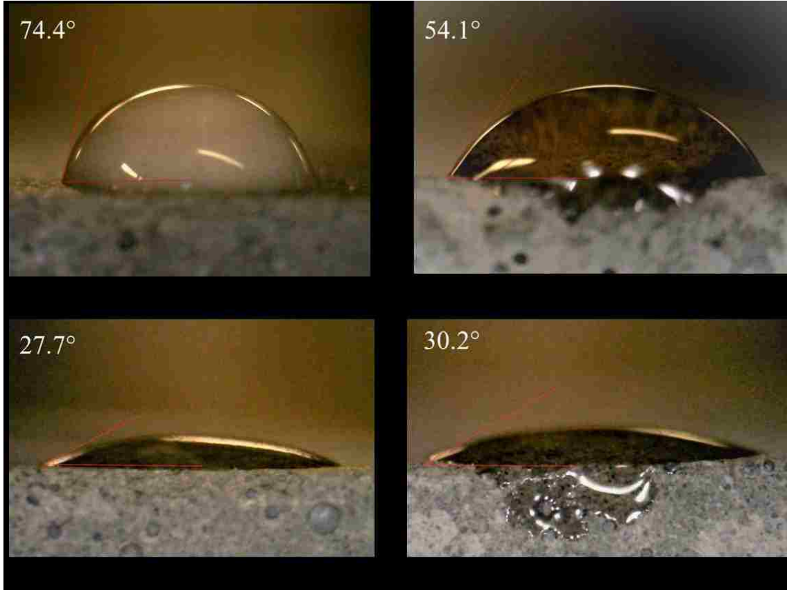
Figure 3.36: Contact angle measurements for (a) Microfine cement, (b) Novolac epoxy, (c) MMA, and (d) NM-MMA.
