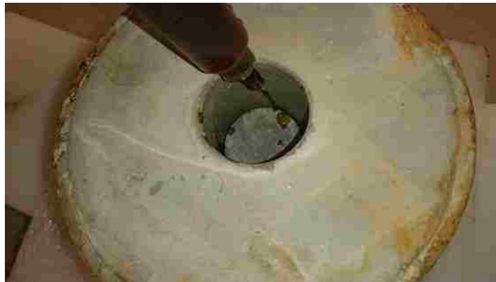
Figure 3.17: Placing seal repair material at the cement-shale microannulus.
