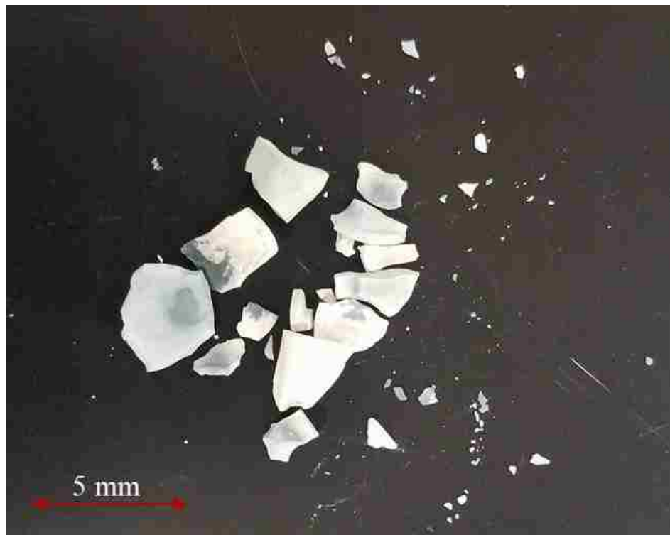
Figure 3.65: Microfine cement fractions falling apart due to harsh environmental conditions.
