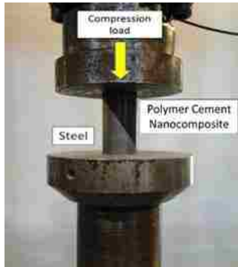
Figure 3.8: Slant shear test setup
