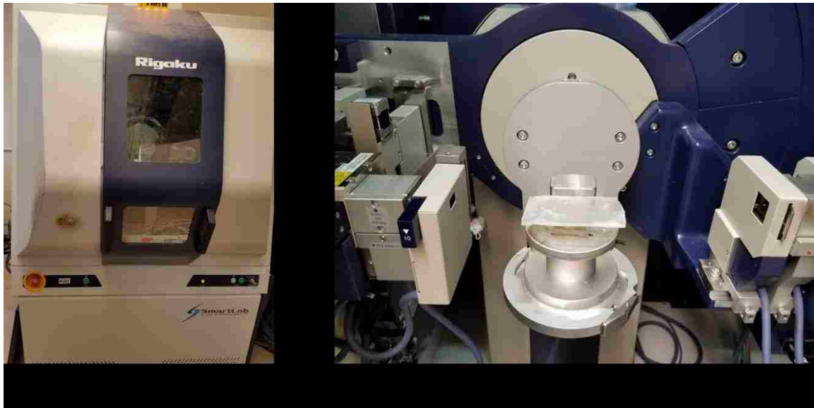
Figure 3.49: (a) Rigaku SmartLab XRD machine and (b) MMA sample on XRD sample holder.
