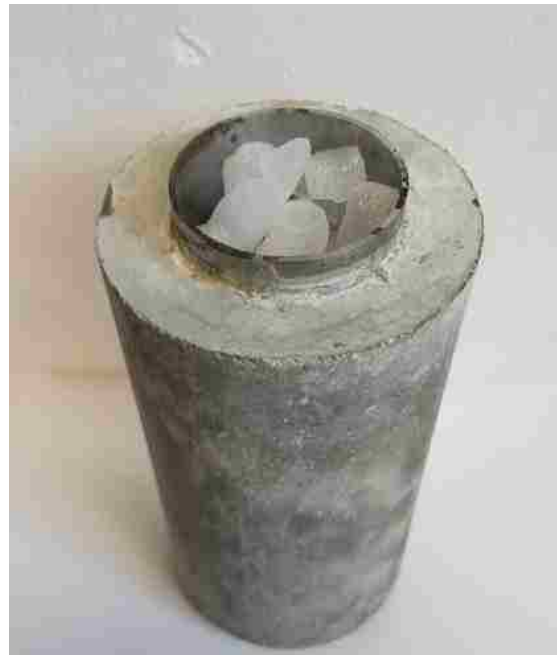
Figure 3.52: Debonding steel casing from the cement sheath using dry ice.
