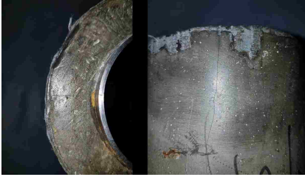
Figure 3.59: Post cyclic test integrated seal specimen sealed with MMA showing a single longitudinal crack in the cement sheath.
