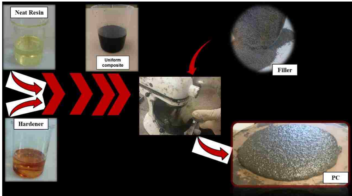
Figure 3.6: Schematic of mixing procedure of polymer-cement nanocomposites.
