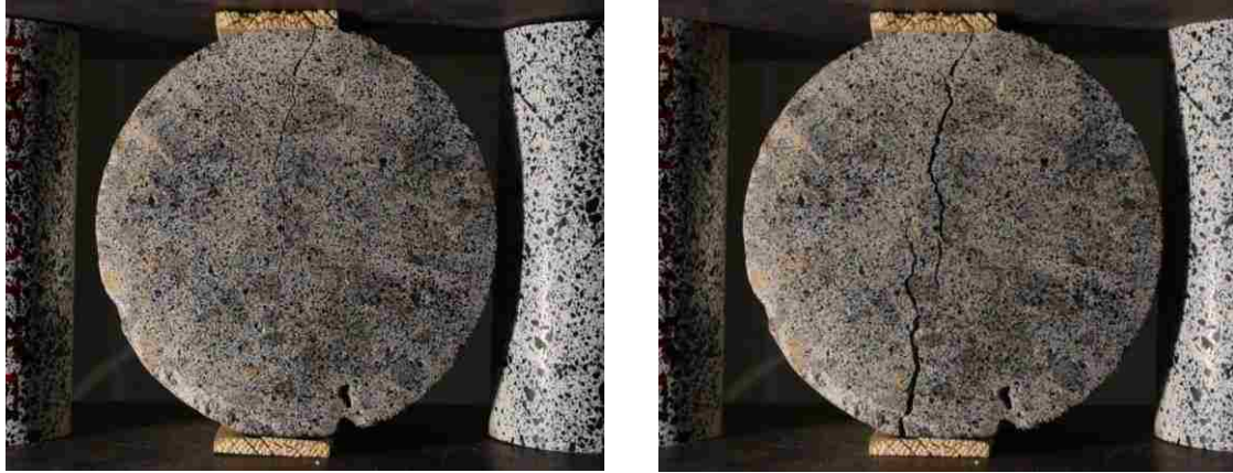
Figure 49: Pre-damaged specimen at beginning and end of test
