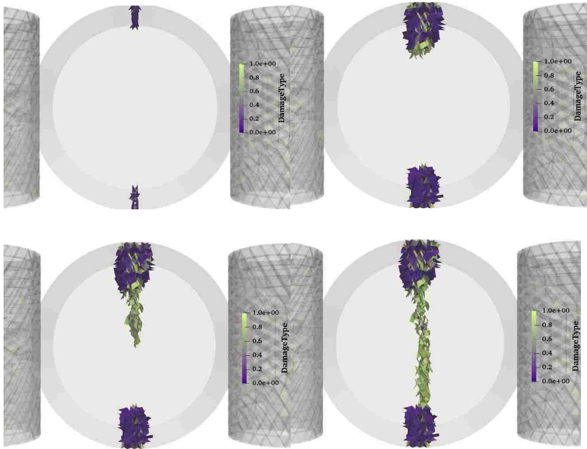
Figure 74: Model damage type progression stiff BITT
