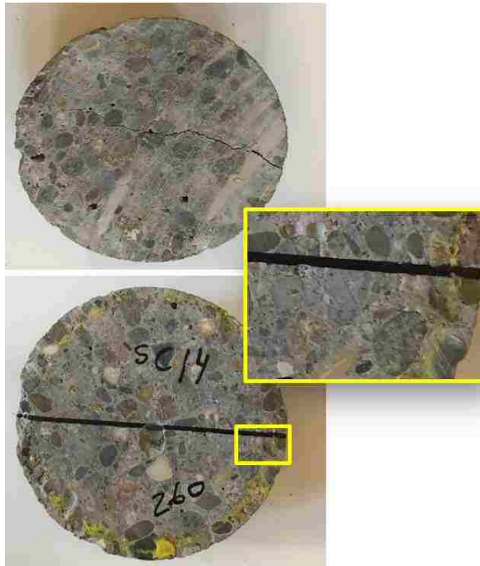
Figure 48: Specimen No. 3 resultant hairline fracture
