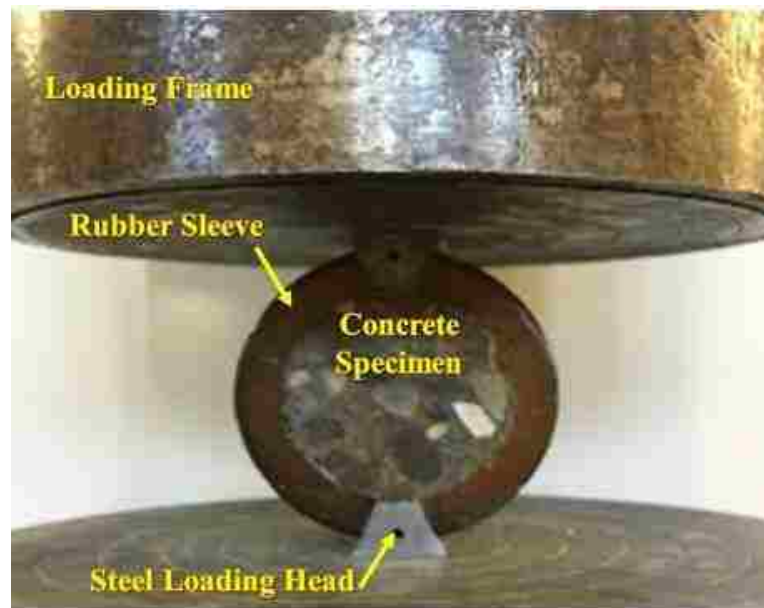
Figure 15: Indirect tension with rubber sleeve
