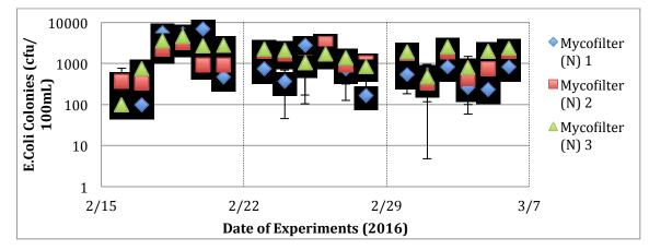
Figure 10: Mycofilter (N) Reactor Results, E. Coli concentrations as a function of time for the mycofilter (N) treatment reactor
