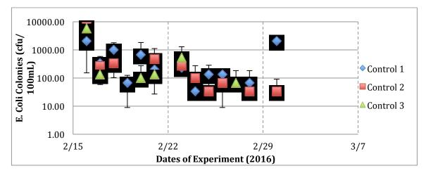
Figure 4: Control Reactor Results, E. Coli concentrations as a function of time for the control treatment reactor with Standard Deviation (+/-)
