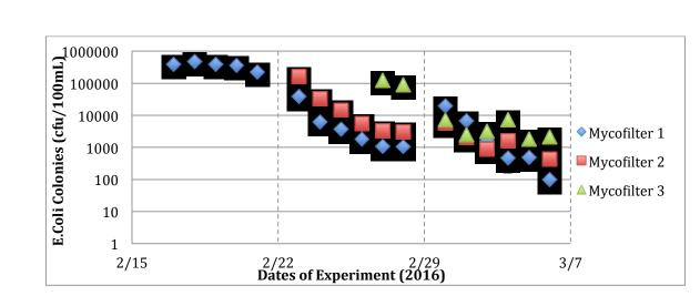
Figure 8: Mycofilter Reactor Results, E. Coli concentrations as a function of time for the mycofilter treatment reactor with Standard Deviation (+/-)
