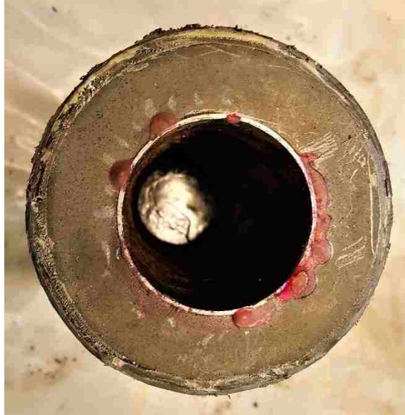
Figure 6. Bottom of a sample after injection, which shows that the epoxy entered the microannulus at the top, flowed through and came out of the bottom.
