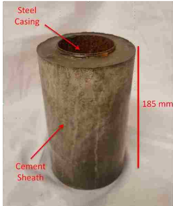
Figure 1. Finished wellbore-shape specimen, comprised of a steel casing and a cement sheath.
