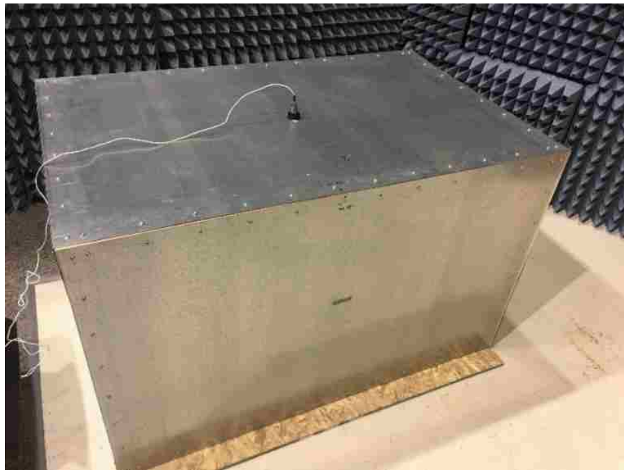
Fig. 6.2. Experimental setup to measure free vibration of the roof with an accelerometer.
