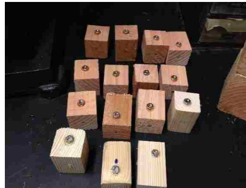
Figure 3-5: Wooden Block Used to Attach Accelerometer
