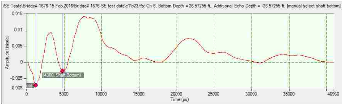
Figure 5-19: Velocity Trace of SE Test No. B23 Using Soft Tip- Wooden Block
