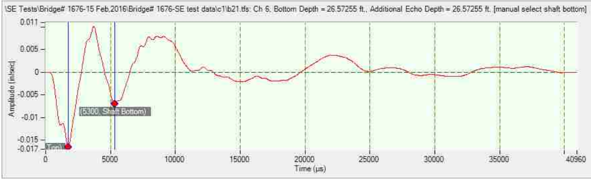
Figure 5-17: Velocity Trace of SE Test No. b21 Using Medium Hard Tip- Wooden Block
