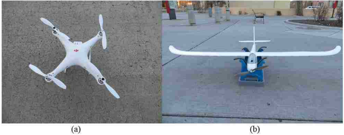
Figure 7. Examples of untethered low altitude AGL S-UAS; (a) rotary-wing S-UAS; (b) Fixed-wing S-UAS
