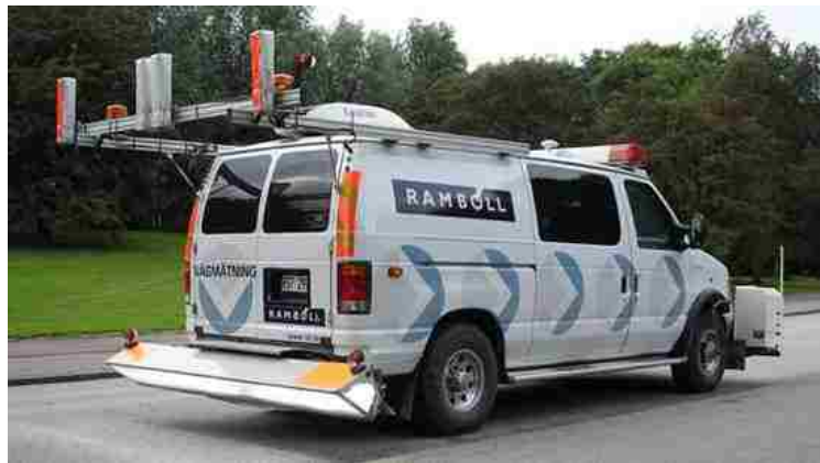
Figure 4. Automatic pavement surface distress evaluation system.
