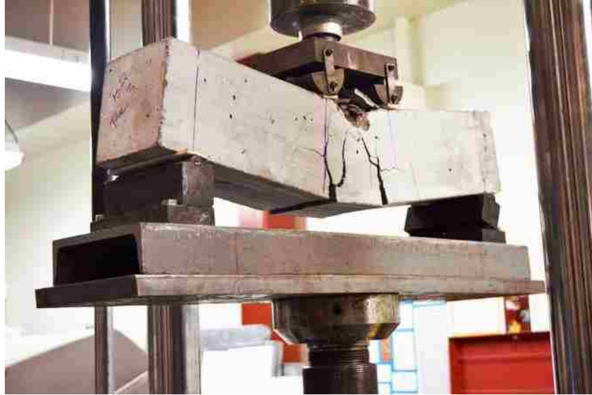
Figure 4.11 Control beam C-3 after failure showing concrete crushing
