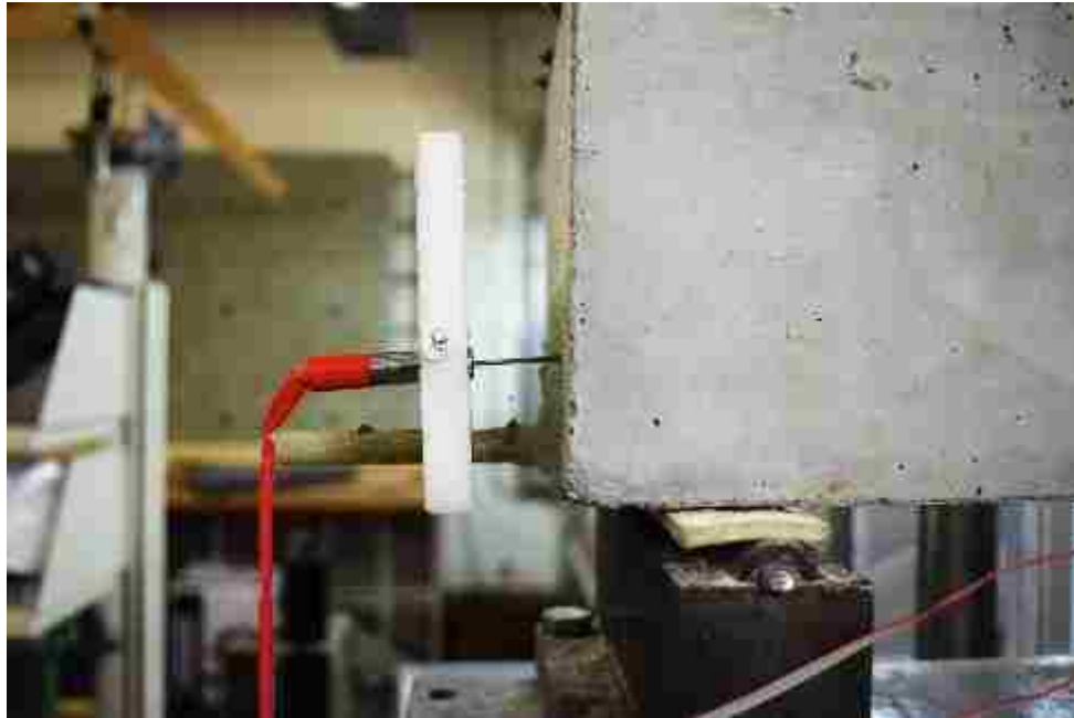
Figure 3.17: LVDT fixture to measure NSM bar debonding
