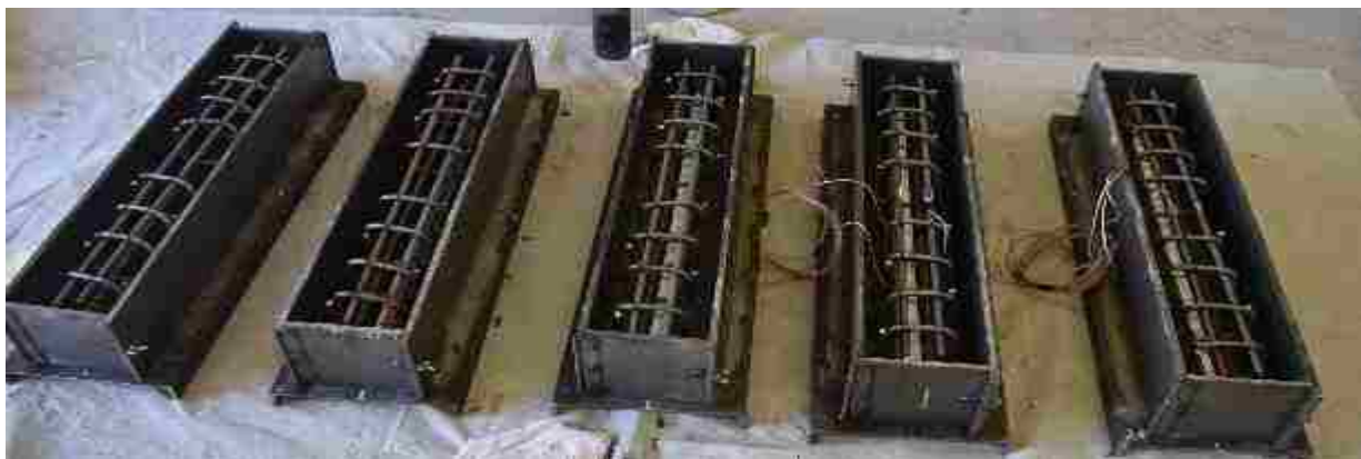
Figure 3.5: Prepared molds before pouring concrete
