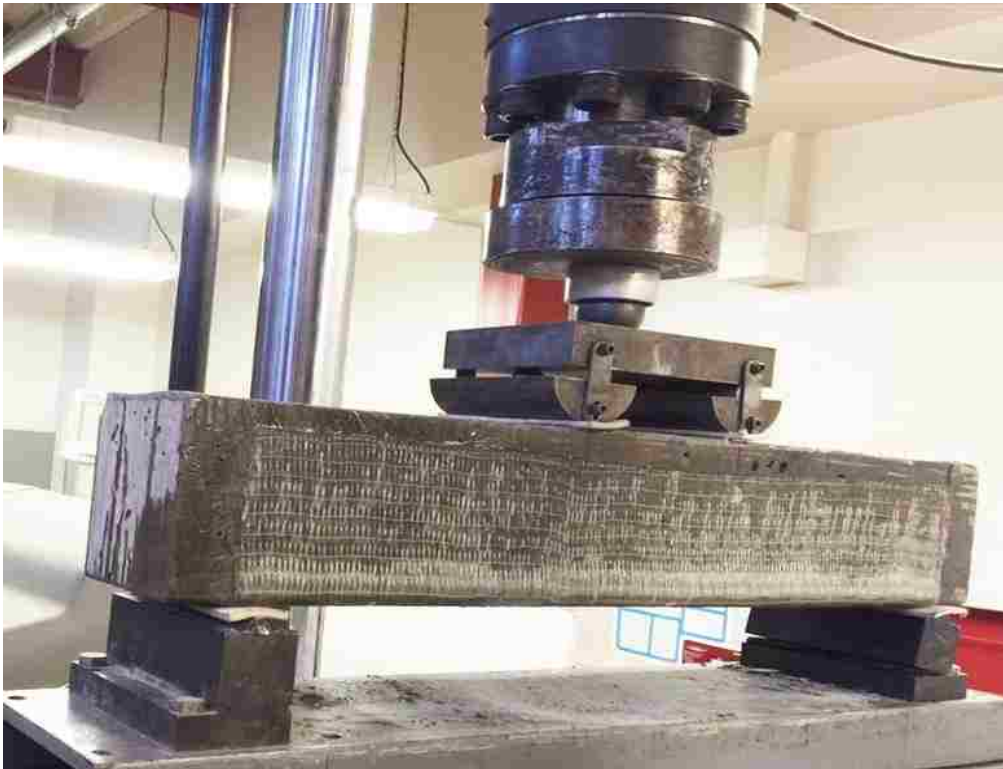
Figure 4.14: FRP U-wrapped beam (U) while loading
