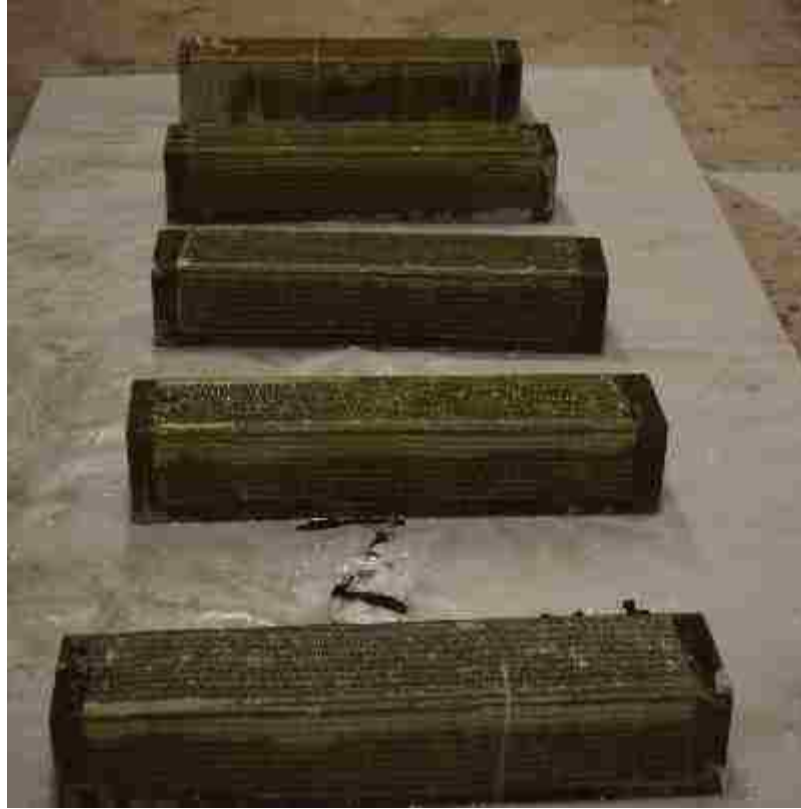
Figure 3.20: Beams with U-wrap shear strengthening only U1-U5 before testing
