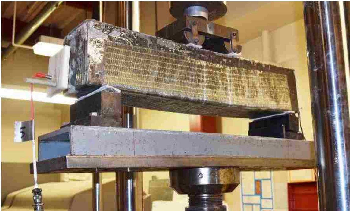
Figure 4.31: RC Beam flexurally strengthened with NSM-FRP and shear strengthened with U-wrap FRP Showing flexural cracks while loading of the beam
