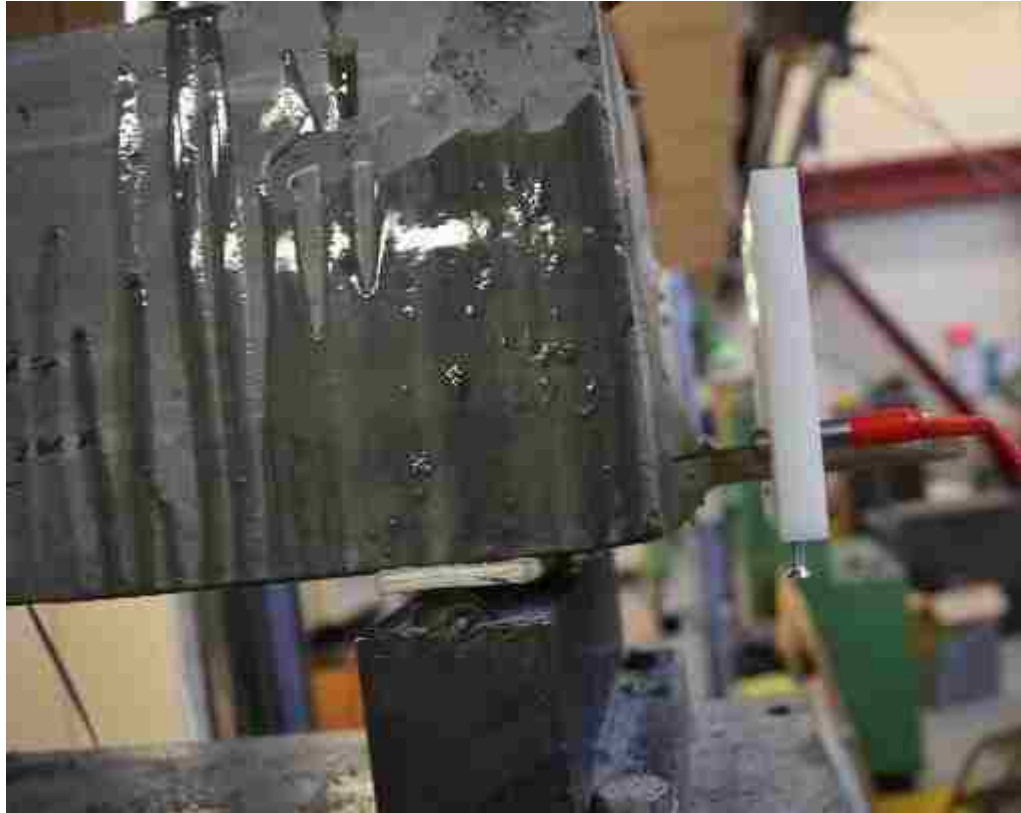
Figure 3.18: LVDT fixture while test in progress showing slip of NSM GFRP bar
