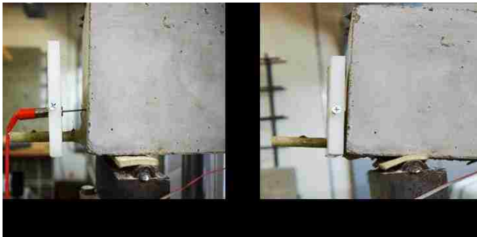
Figure 4.28: NSM-GFRP bar slip (a) before failure (b) after failure
