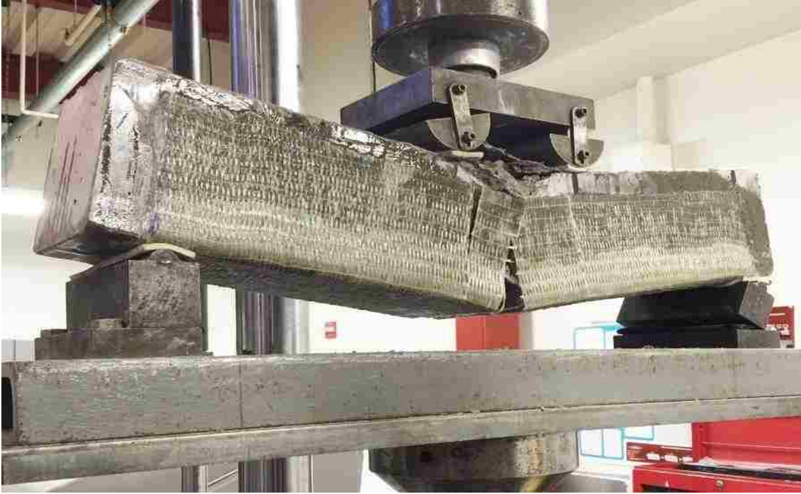
Figure 4.16: RC Beam U3 after failure
