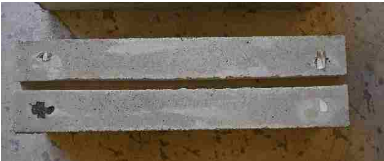
Figure 3.7: Beam NSM groove after cleaning
