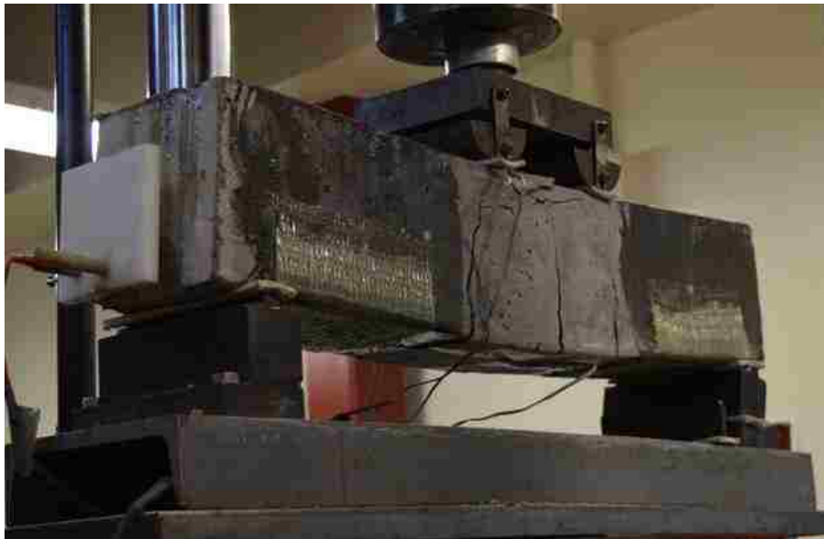
Figure 4.48: RC Beam flexurally strengthened with NSM-FRP and shear strengthened with U-wrap FRP in shear area only after failure
