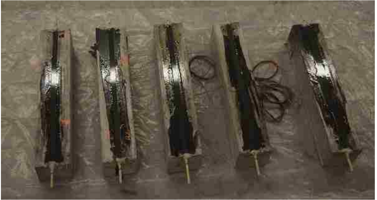
Figure 3.21: Beams with NSM flexural strengthening only N1-N5 before testing
