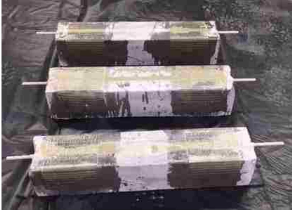
Figure 3.23: Beams with NSM flexural strengthening and U-wrap shear strengthening in shear zone only NUS2-NUS4 before testing, where NUS1 was already tested
