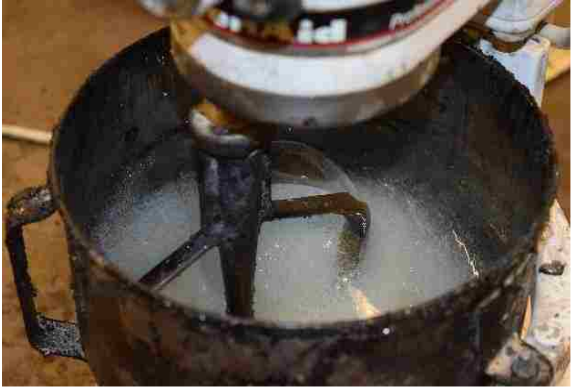
Figure 3.12: Mixing of epoxy for wet-layup
