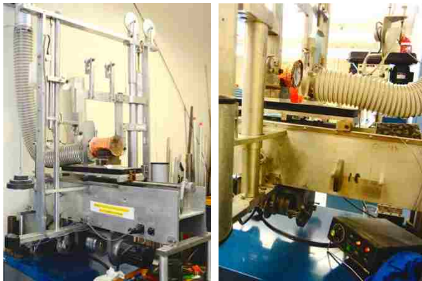
Figure A-6: Diamond wire saw with ventilation, pulley system, adjustable table, wheel, pump and pump controller.
