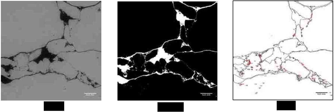
Figure 2: a. Original BSE-SEM image. b. Threshold of image adjusted with white pore space and black grain space. c. Generated outline of counted pores after particles were analyzed.
