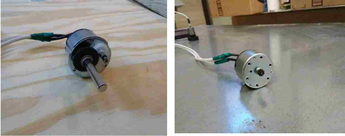
Figure 6.10: a) DC gear motor without the off-balance rotating mass b) DC motor without the off-balance rotating mass and gear system
