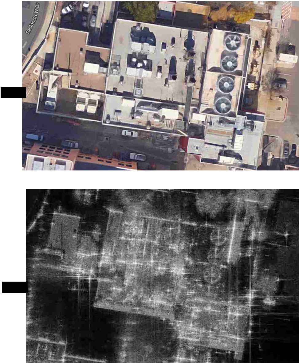
Figure 1.1: a) Google image of the roof of Ford Utility Building. b) SAR image of the roof of the Ford Utility Building
