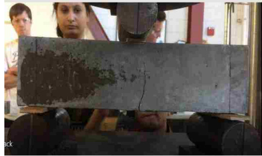
Figure b: Initiation of crack; back face
