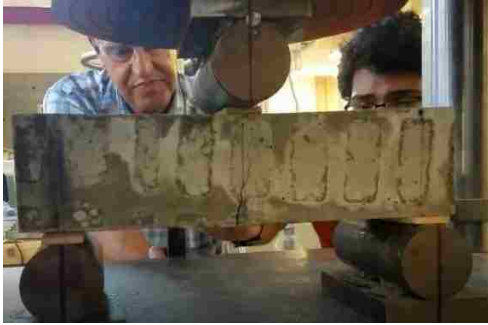
Figure a: Initiation of crack; front face
