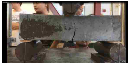
Figure d: Final crack; back face
