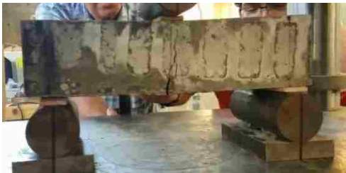
Figure c: Final crack; front face
