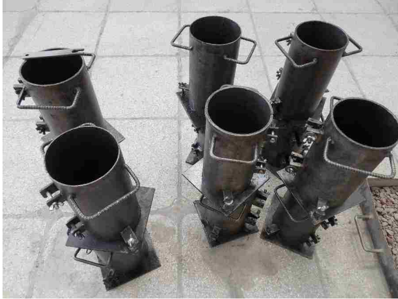
Metallic cylindrical molds
