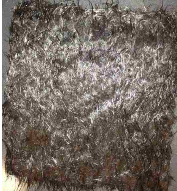
Figure 15. Recycled carbon fiber mat
