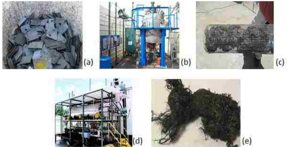
Figure 12. Recycling carbon fiber composite at Adherent Technologies, Inc. (a) composite plates prior to recycling (b) reactor of wet chemical composite (c) carbon fiber extracted from the reactor (d) Vacuum furnace (e) recycled carbon fibers
