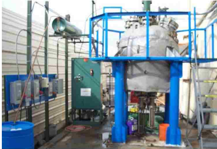
Figure 9. Low temperature, Low pressure recycling reactor
