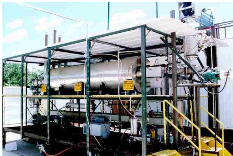
Figure 8. ATI's Phoenix reactor, a pilot scale vacuum pyrolysis unit[8]
