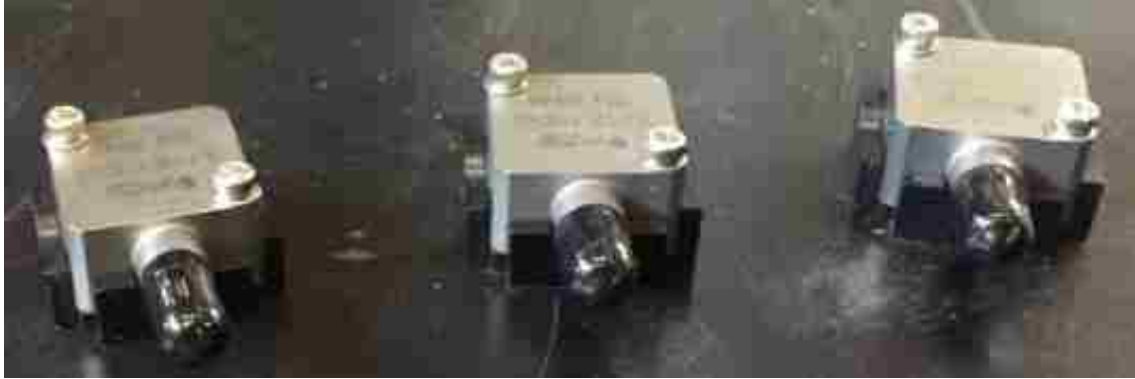
Fig. 3.5. 3711B110G accelerometers close-up.
