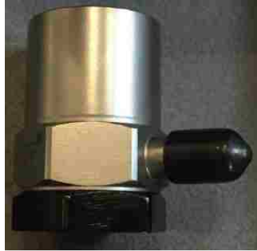
Fig. 4.1. 353B33 ICP accelerometer close-up.
