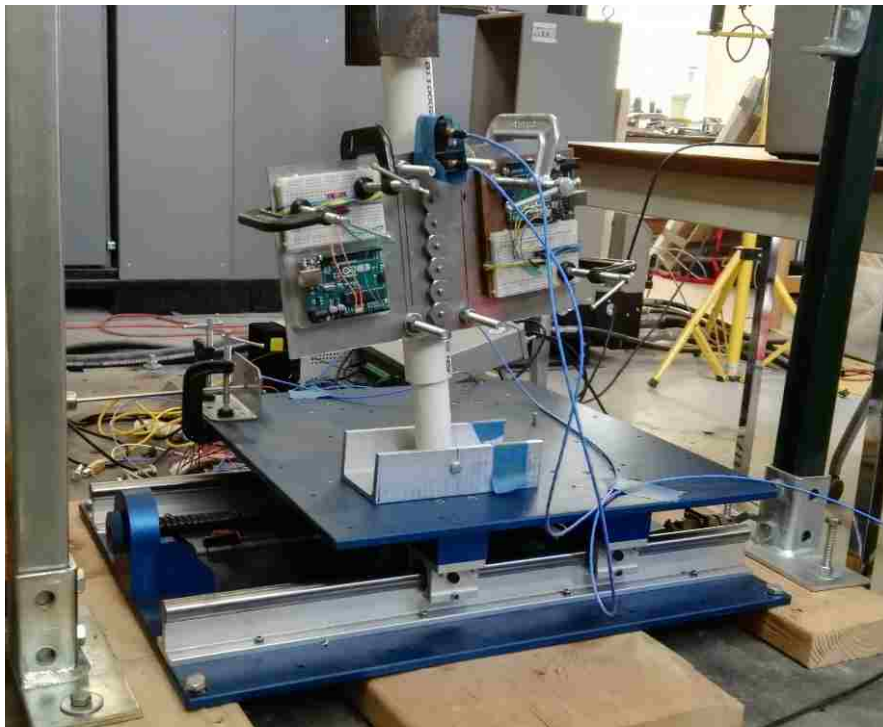
Fig. 5.3. Low-cost tilt measurement estimation set-up.
