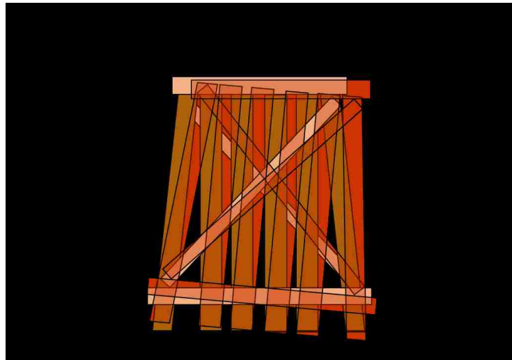
Fig. 3.1. Schematic relation between tilt and displacement of a railroad timber trestle.
