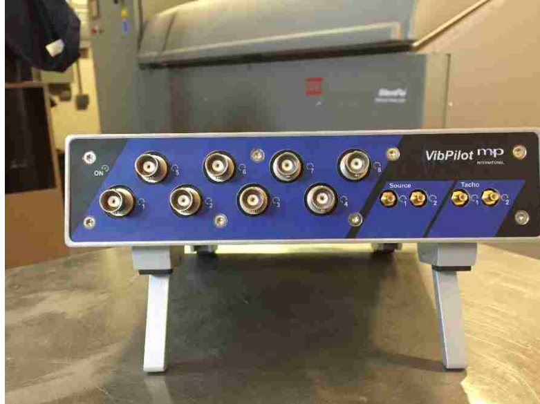
Fig. 3.6. Vibpilot Data Acquisition System.
