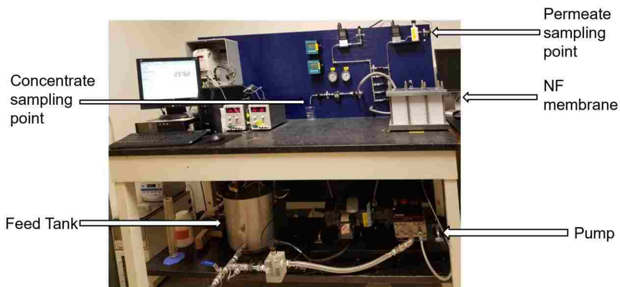
Figure 13: Experimental Setup of RO system for rejection test
