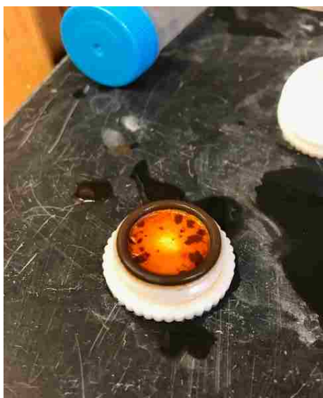
Figure 8: Fe(OH) 3 Filtered by the Pall Corporation Membrane.
