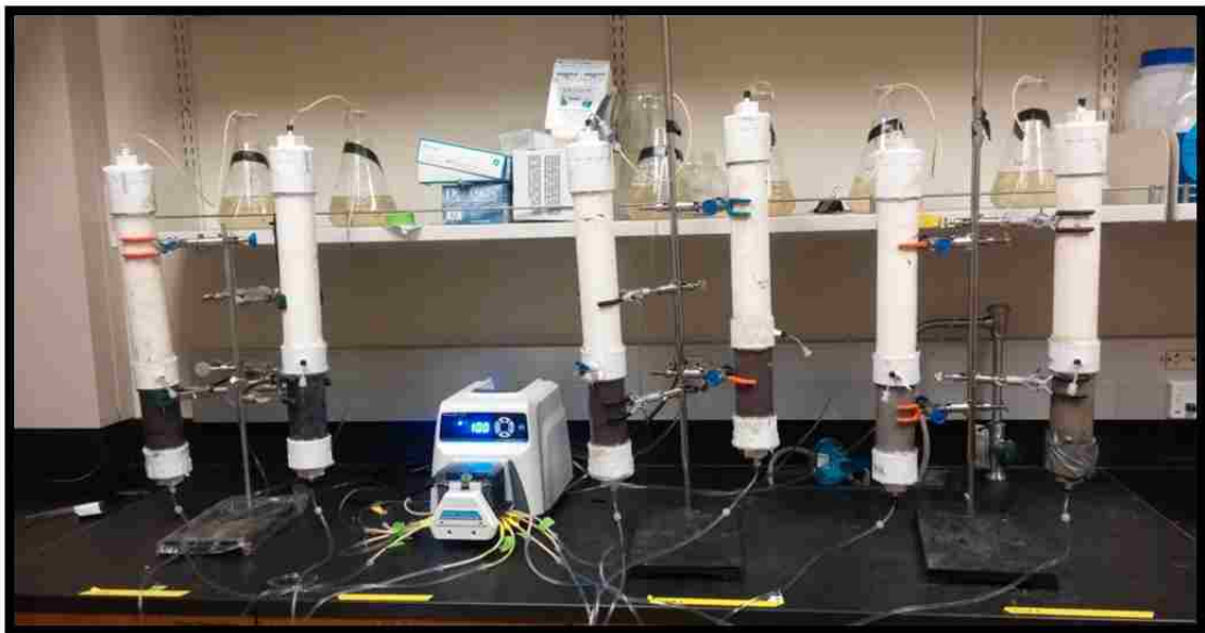
Figure S2. Experimental setup. Six PVC columns packed in two replicates with three different materials 1) gravel, 2) native sediments, and 3) silica sand.
