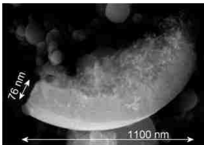
Figure 6.10: SEM image of a particle fragment of NbRu y O z -Dry-Air. During spray pyrolysis or thermal processing, particle surfaces may become nearly impermeable before volatile species can escape to the atmosphere. The pressure developed by these trapped volatiles is sometimes sufficient to fracture some particles.
