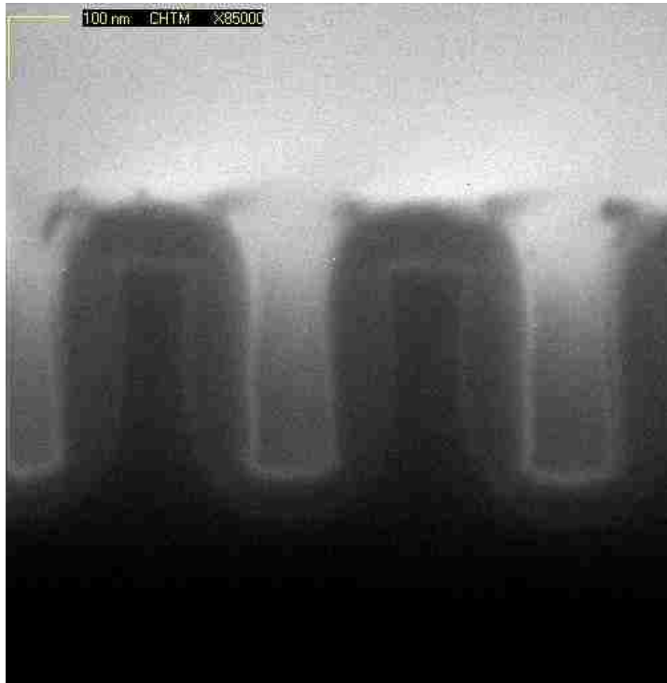
Figure 4-12. A cross-sectional SEM image showing a thick thermally grown oxide layer on the Si channels.
