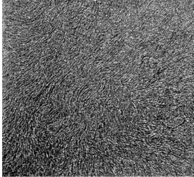
Figure 1-1. Photograph illustrating the textured ordering of Ni platelets observed in a composite in which the magnetic field was applied normal to the plane of the picture.
