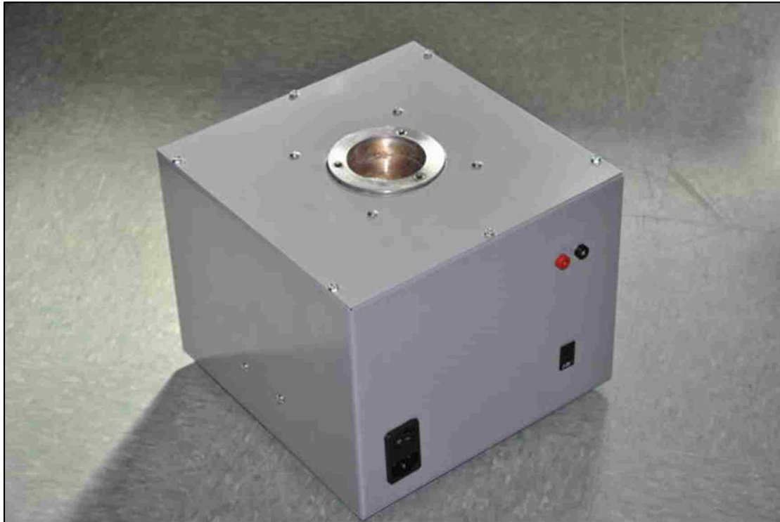
Figure A1-3. The heater block and electronics are contained within a metal housing with ports for temperature and software control.
