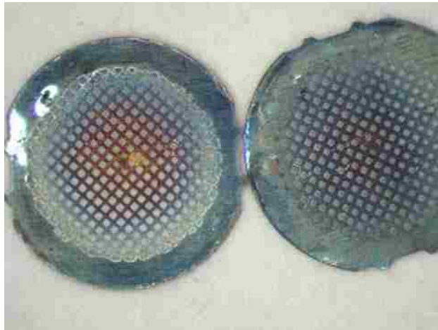
Figure 93 Optical microscope image of TEM grids after experiments of Ni/MgAl 2 O 4 heated to 750°C at 1:1 H 2 :H 2 O 3.6mbar. The left grid is from an experiment using the spacer ring, while the grid on the right used the two 50 mesh grids.
