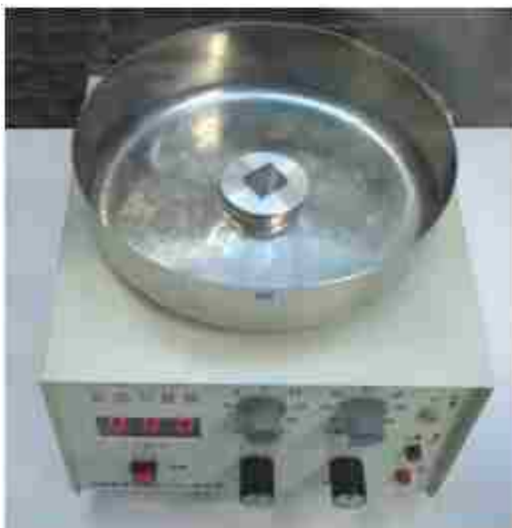
Figure 2.2: Spin coater used for co-depositing pNIPAM with a sol-gel, resulting in spNIPAM films.
