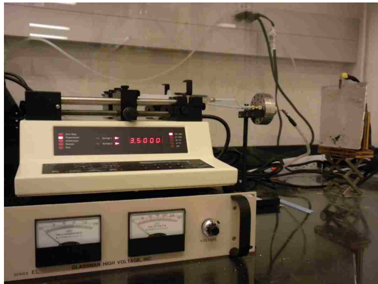
Figure 2.6: Electrospinning setup to produce espNIPAM mats.
