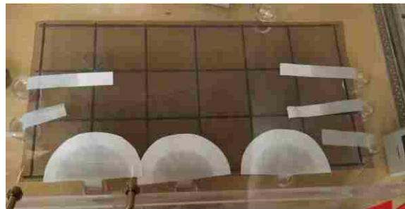
Figure G.2. Laboratory configuration for horizontal wetting experiments.
