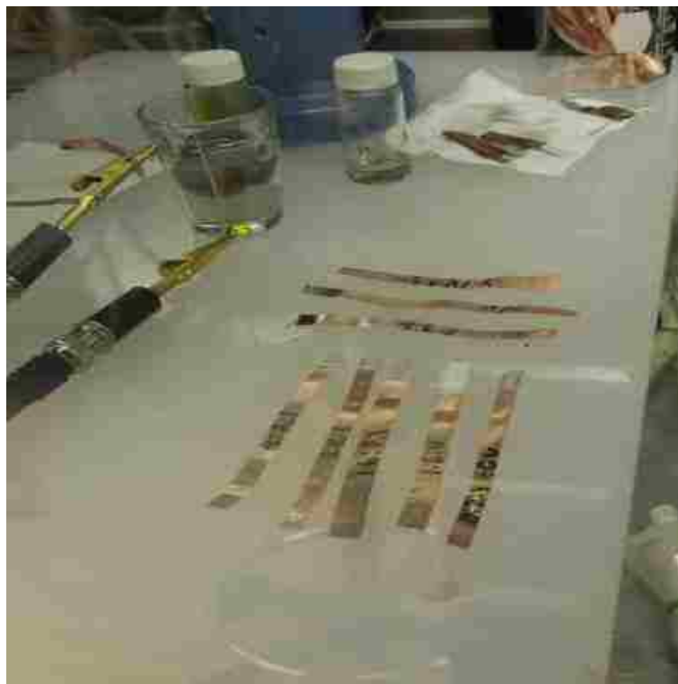
Figure 36: Electrodeposition of Aluminum on Copper from Various Electrolyte baths
