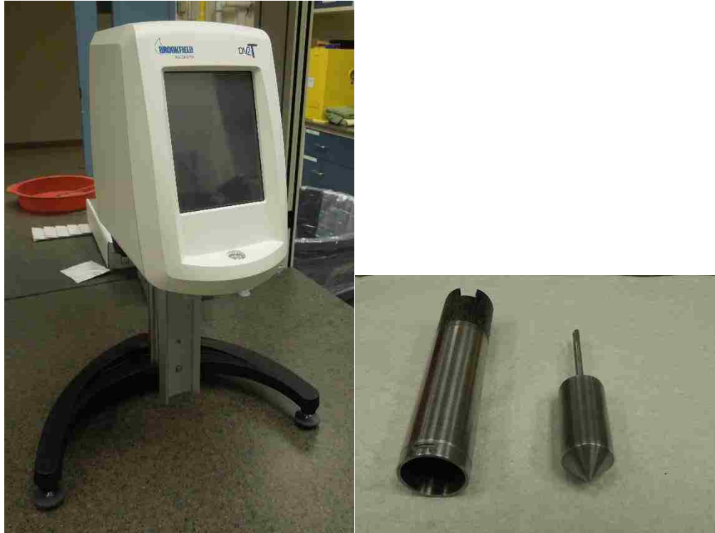
Figure 19: DV2T Programmable Rheometer and y-21 Spindle and Cup Pair with Temperature Probe
