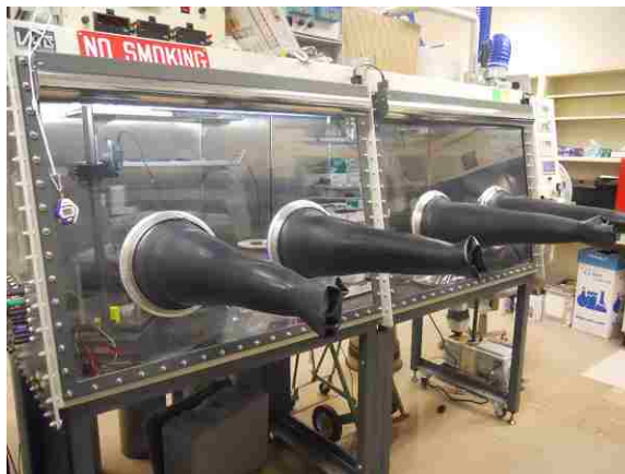
Figure 2.4: Argon glove box used for testing.
